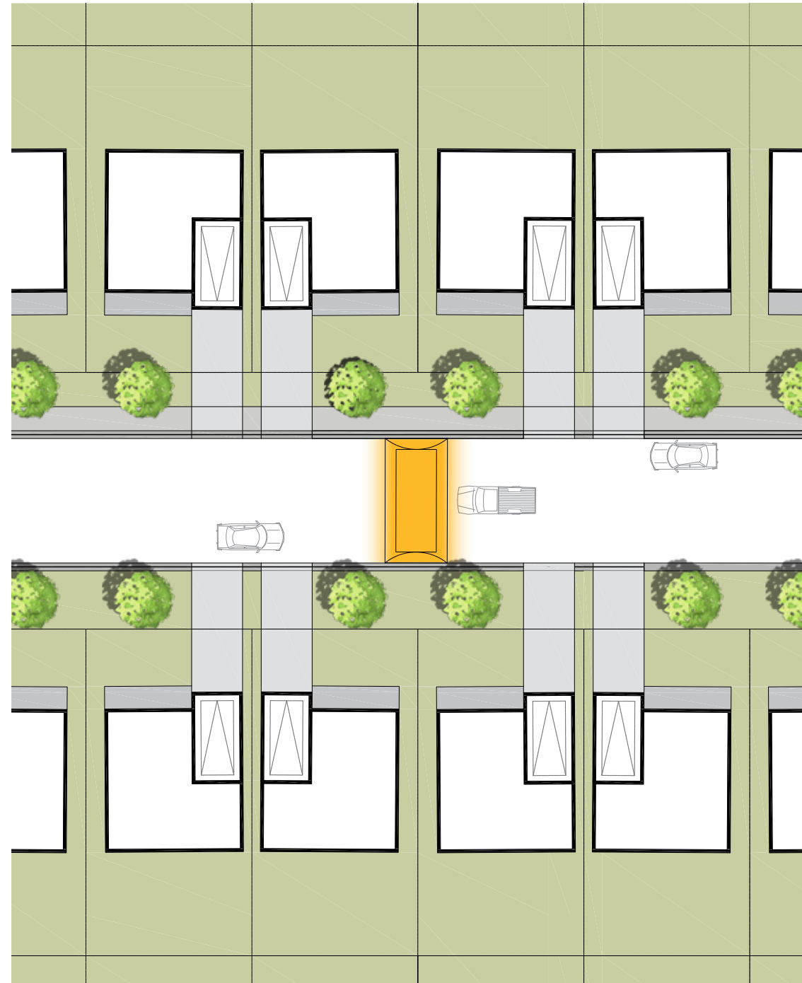
Figure 32 Speed Hump on Local Street
