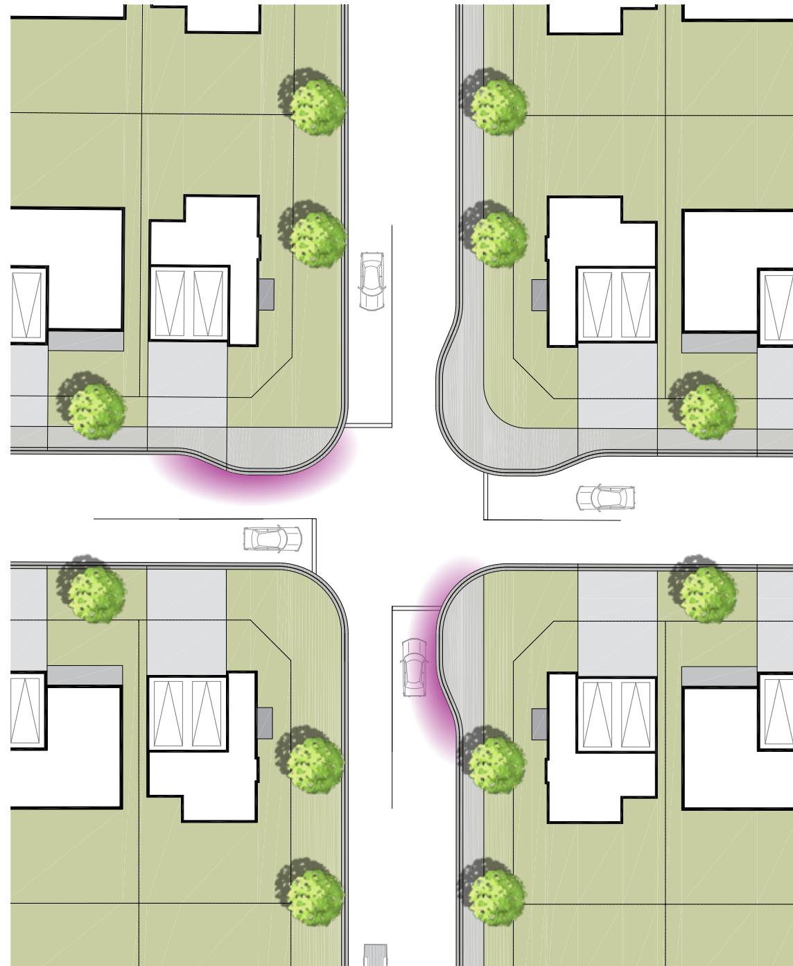
Figure 30 Single Bulb-Out at Intersection
