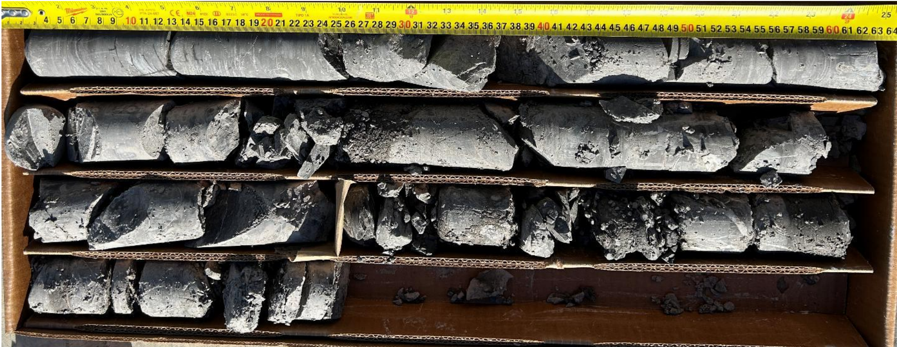
BH105-25 Cored length 5.69 to 7.85 mbgs Core Box 2 of 2
