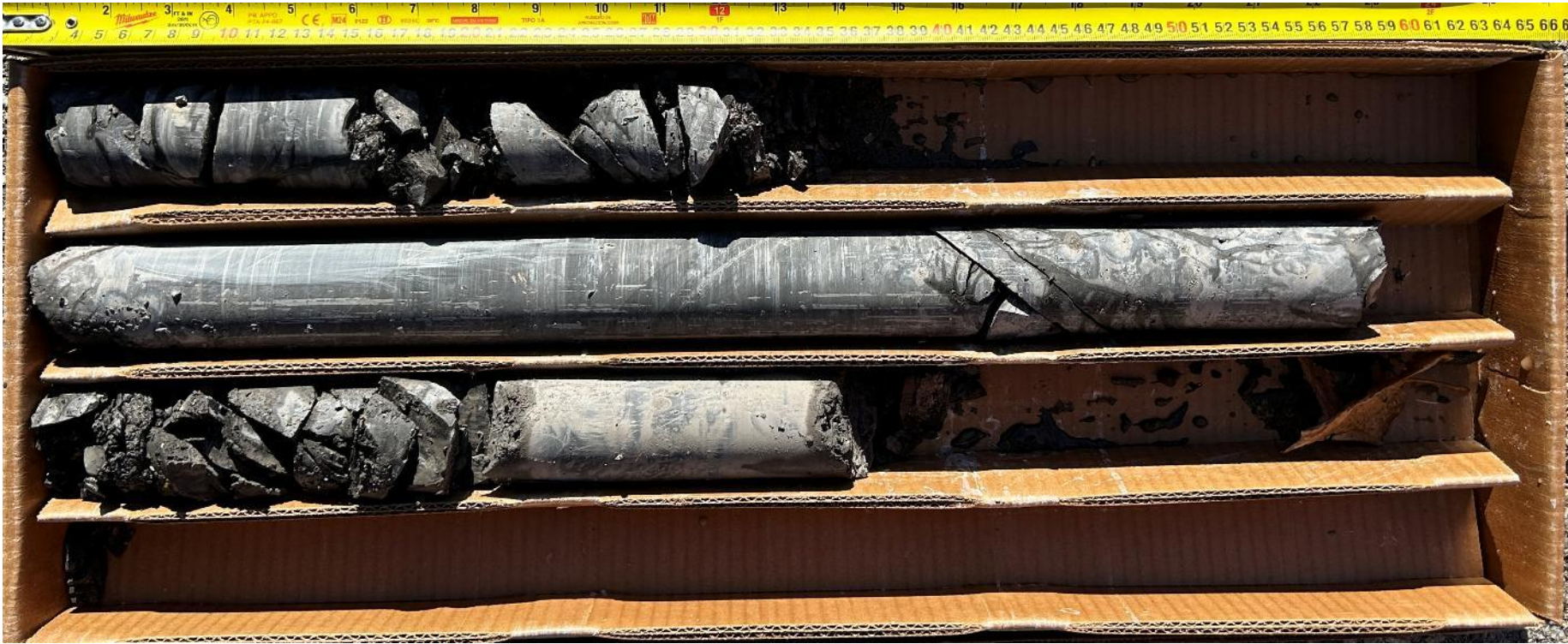
BH103-25 Cored length of 7.09 to 8.59 mbgs Core Box 2 of 2
