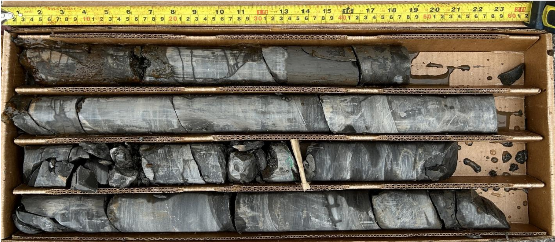
BH101-25 Cored length of 2.57 to 4.75 mbgs Core Box 1 of 3
