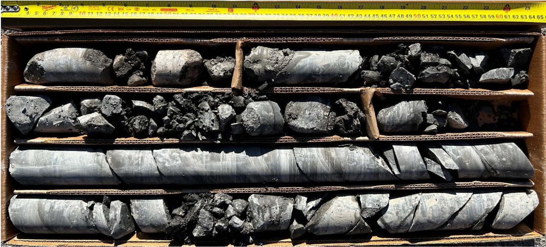
BH103-25 Cored length of 2.23 to 7.09 mbgs Core Box 1 of 2
