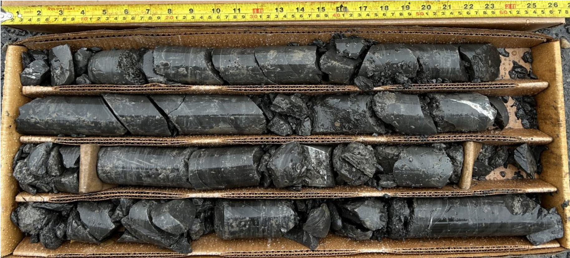
BH102-25 Cored length of 2.39 to 6.22 mbgs Core Box 1 of 2
