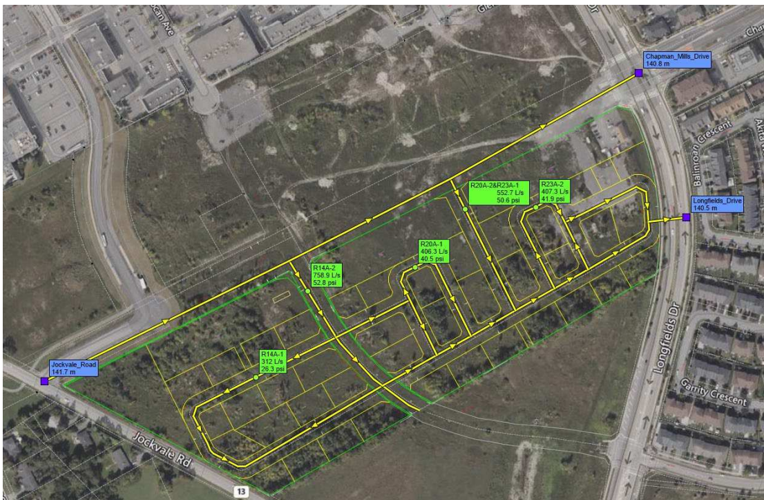
Figure 3.9: Available Fire Flows (L/s) During MXDY Condition Before SUC Pressure Zone Reconfiguration
