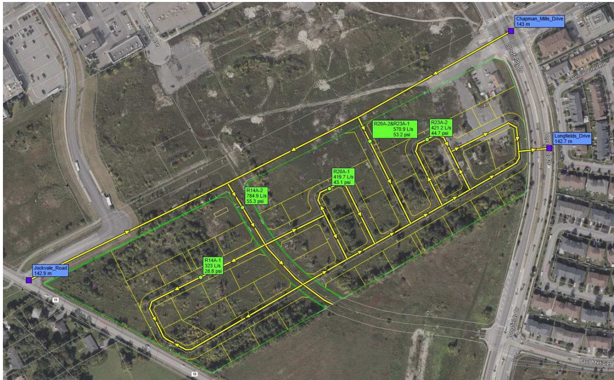
Figure 3.10: Available Fire Flows (L/s) During MXDY Condition after SUC Pressure Zone Reconfiguration
