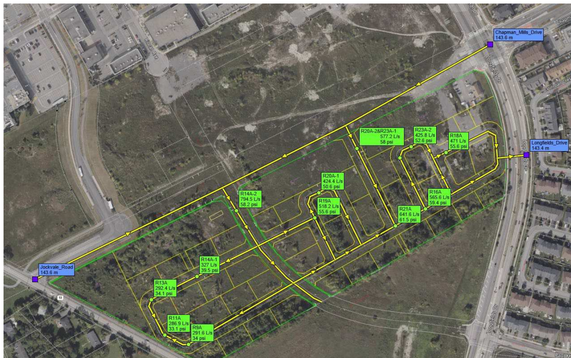
Figure 3.8 Available Fire Flows (L/s) During MXDY Condition After SUC Pressure Zone Reconfiguration
