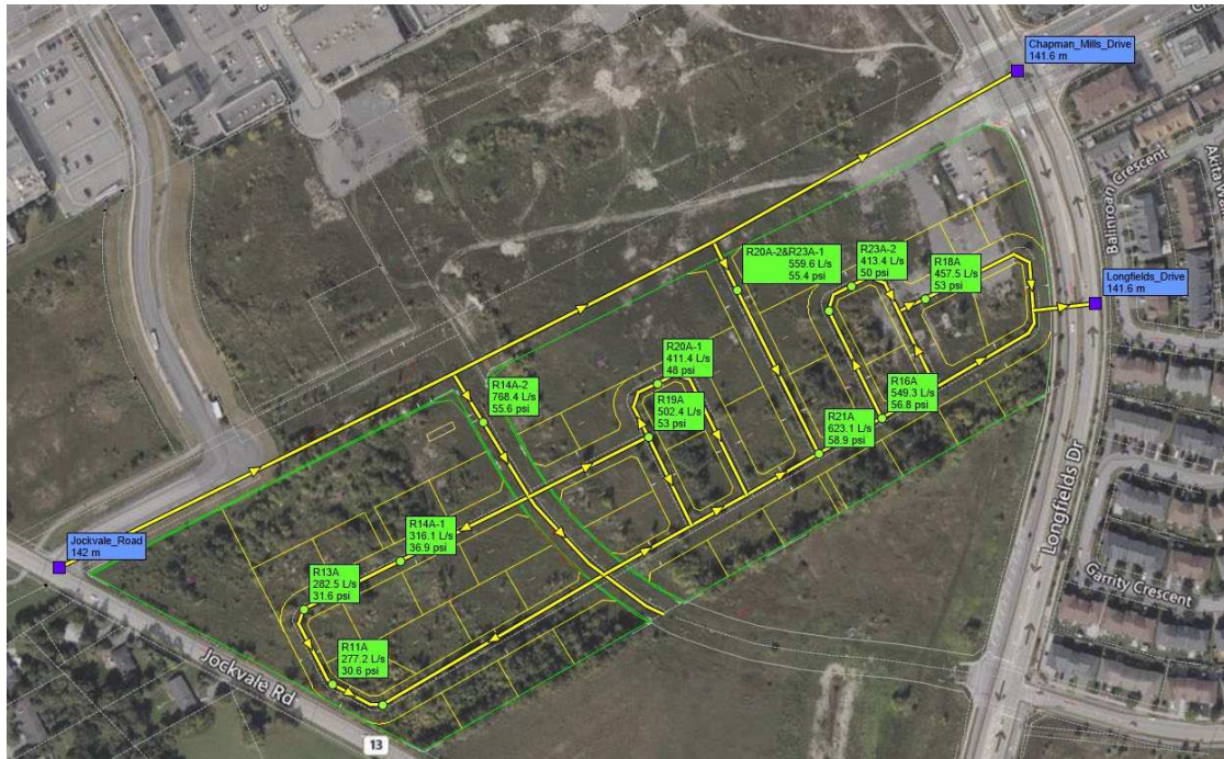
Figure 3.7 Available Fire Flows (L/s) During MXDY Condition Before SUC Pressure Zone Reconfiguration
