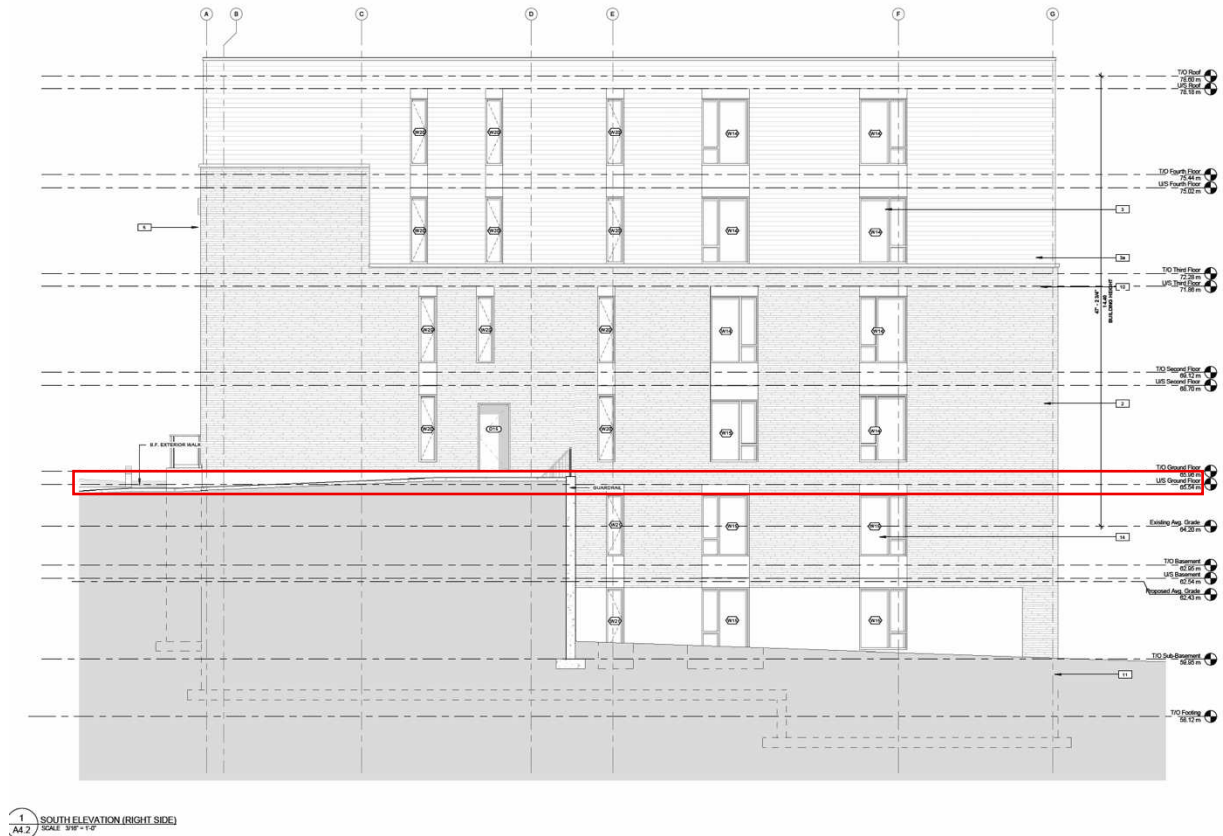
Figure 3: 3D South Elevation with average grade shown in red (Source: Lawrence Architects)
