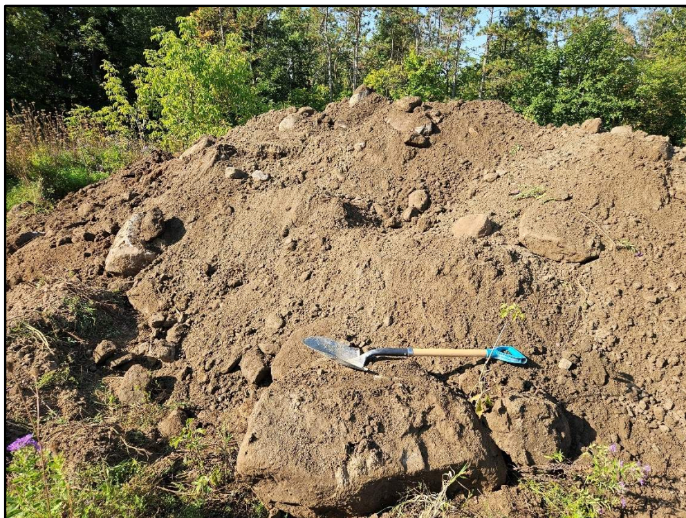
Photo 6: Photo illustrating the boulders excavated from the test pit TP 3-24.
