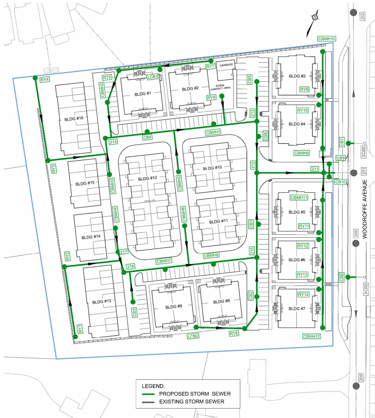
Figure 5: Storm Sewer Network
