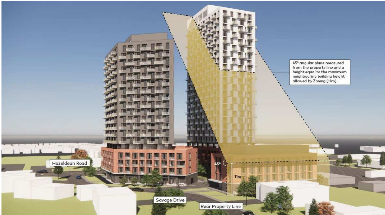
Figure 15: 45-degree angular plane, measured from the rear lot line (Source: Figurr Architects)
