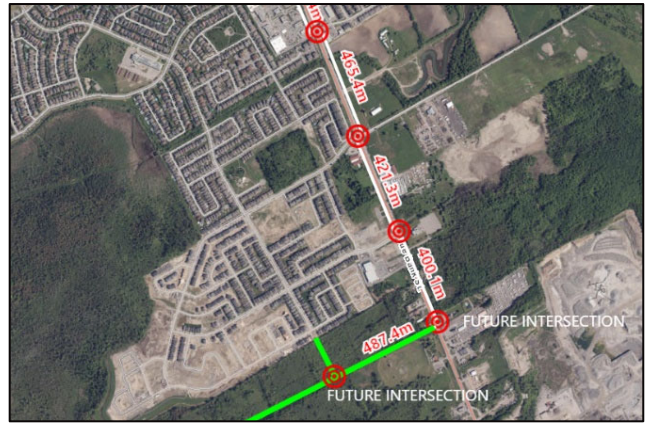
Figure 8 - Arterial Road Intersection Spacing
