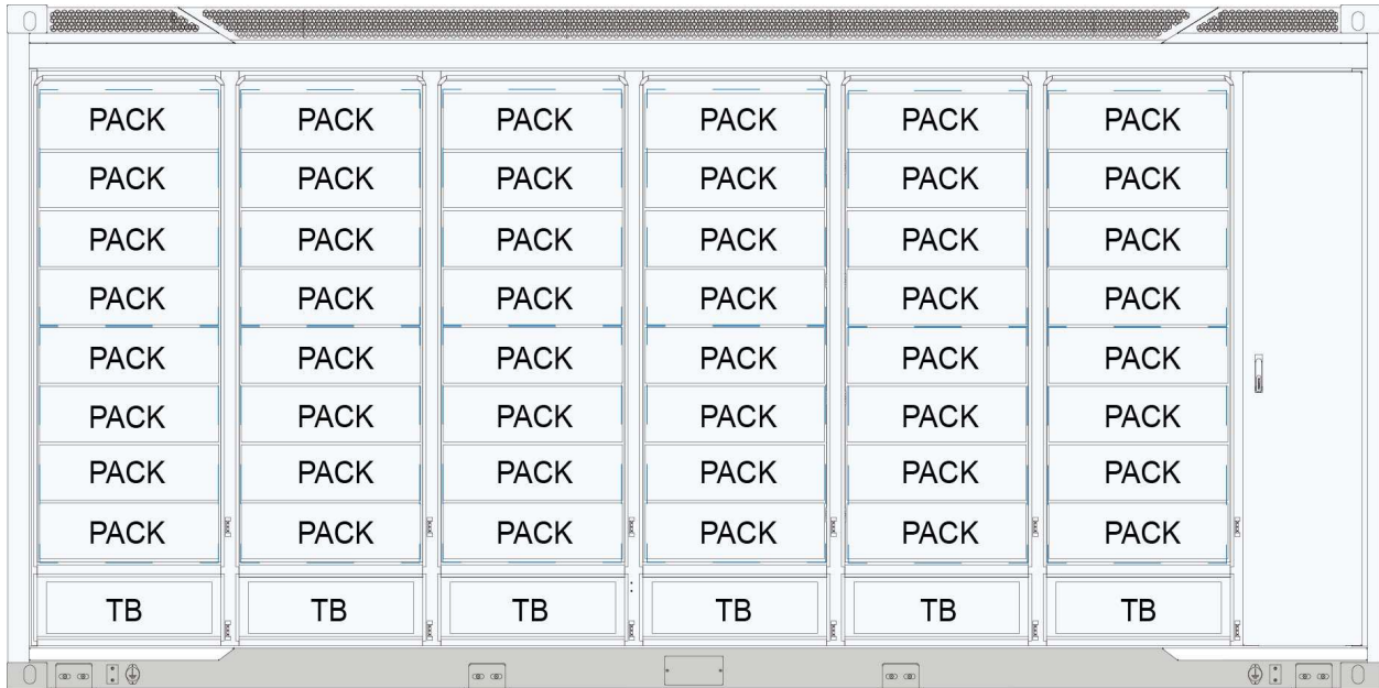
Figure 4 - Example Battery Stack Configuration
