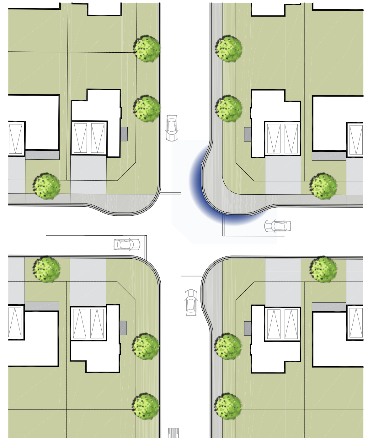
Figure 40 Double Bulb-Out at Intersection
