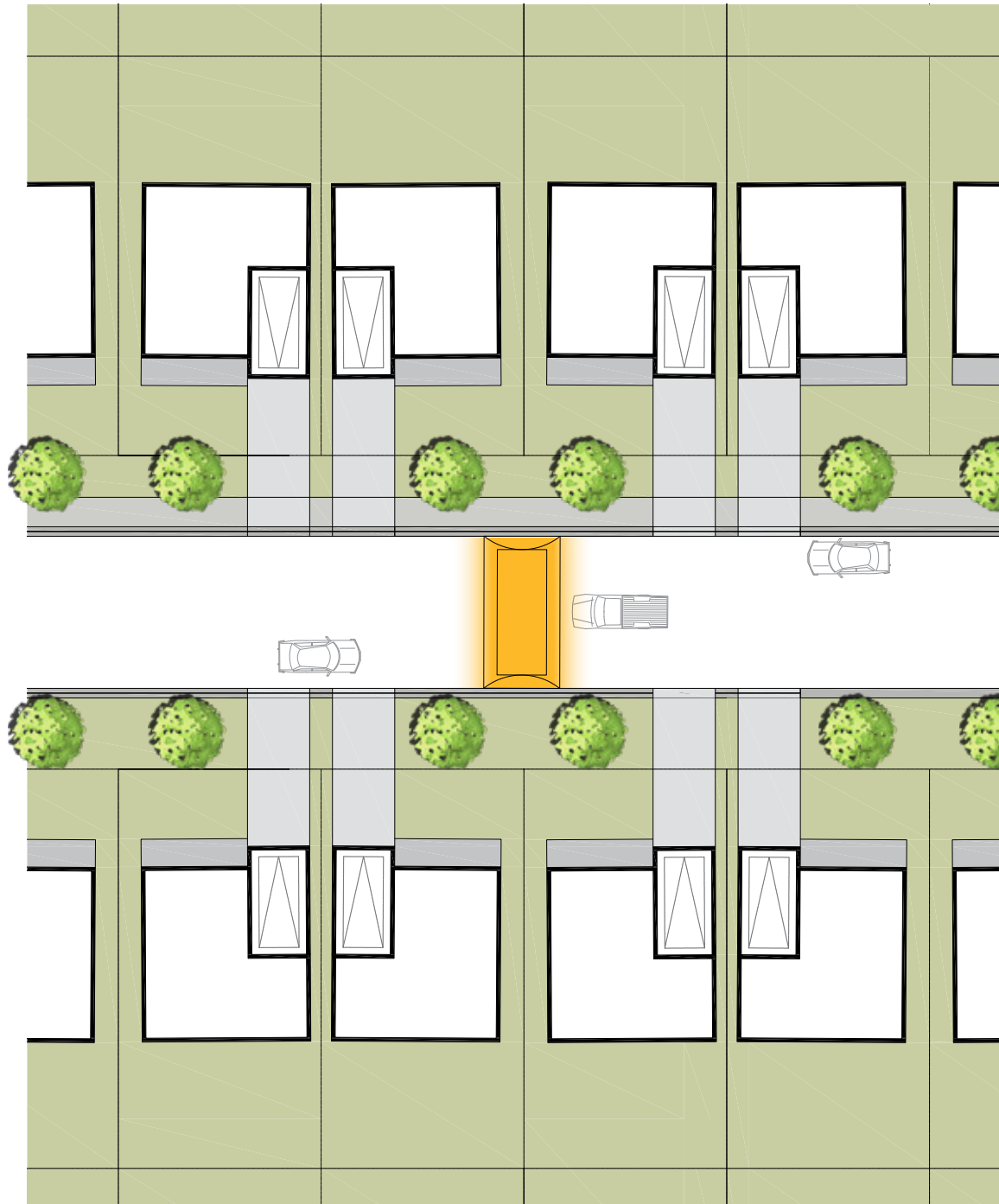
Figure 41 Speed Hump on Local Road
