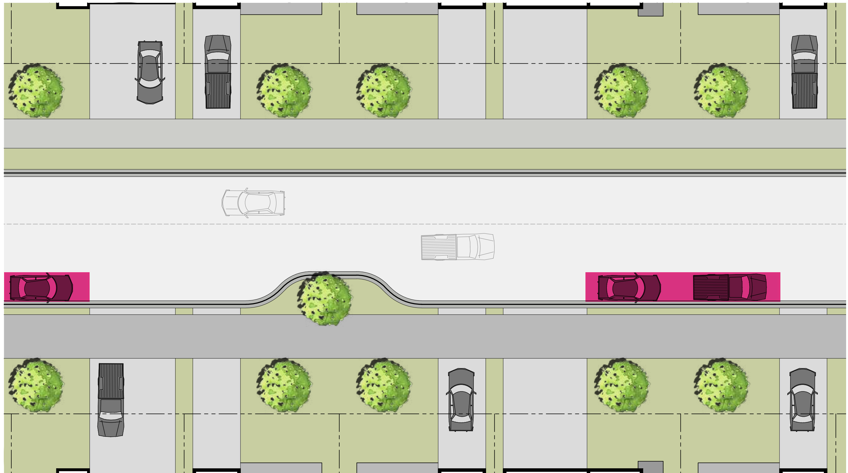
Figure 35 On-Street Parking Demonstration on Collector Road
