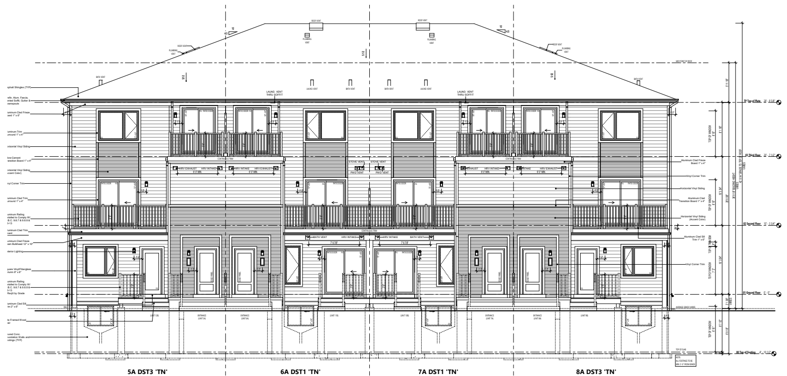
Rear Elevation of a 12 unit back-to-back townhouse. (Prepared by Bim Studio + Organica Studio.)
