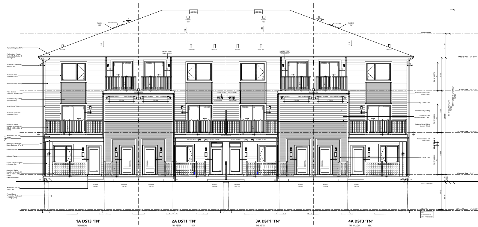
Front Elevation of a 12 unit back-to-back townhouse. (Prepared by Bim Studio + Organica Studio.)
