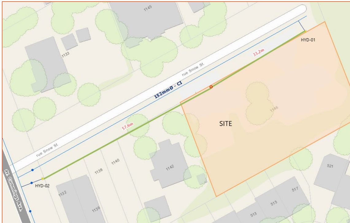
Figure 3.1: Fire Hydrant Coverage Sketch
