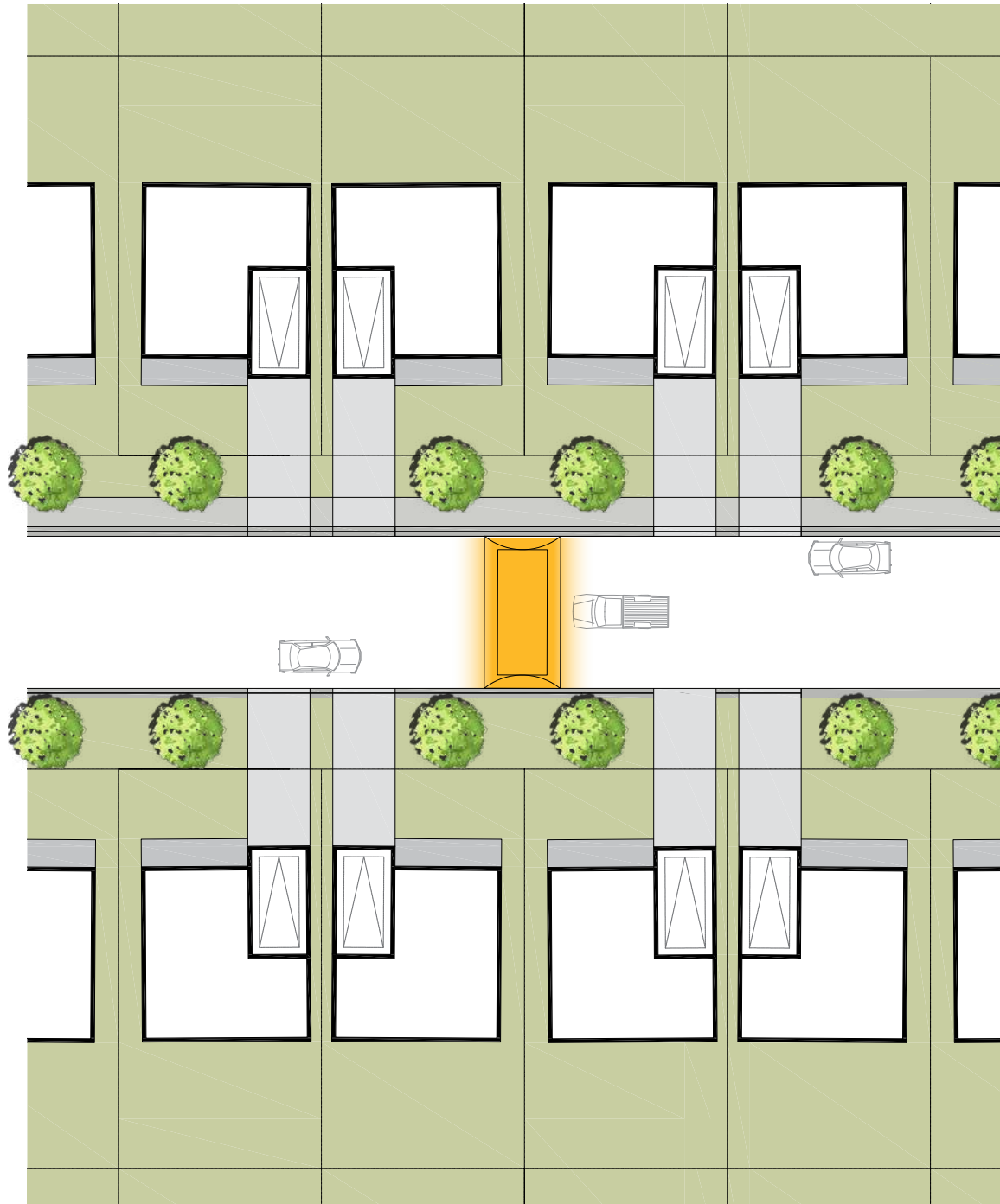
Figure 40 Speed Hump on Local Road
