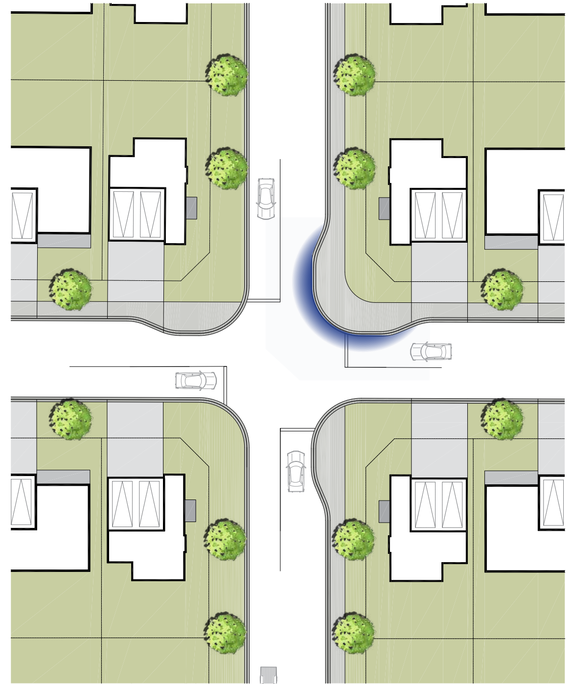
Figure 39 Double Bulb-Out at Intersection
