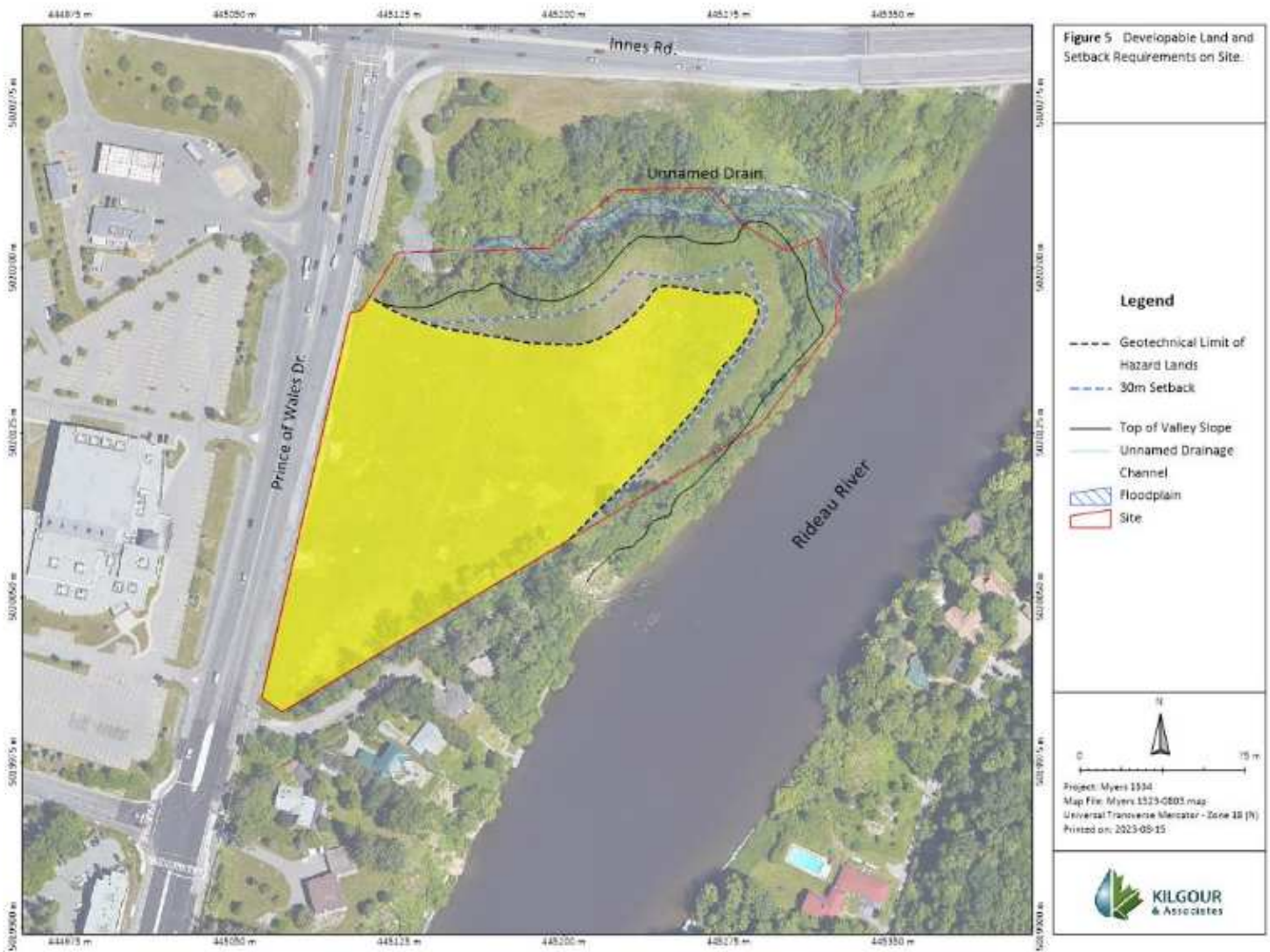
Figure 5 Developable Land and Setback Requirements on Site
