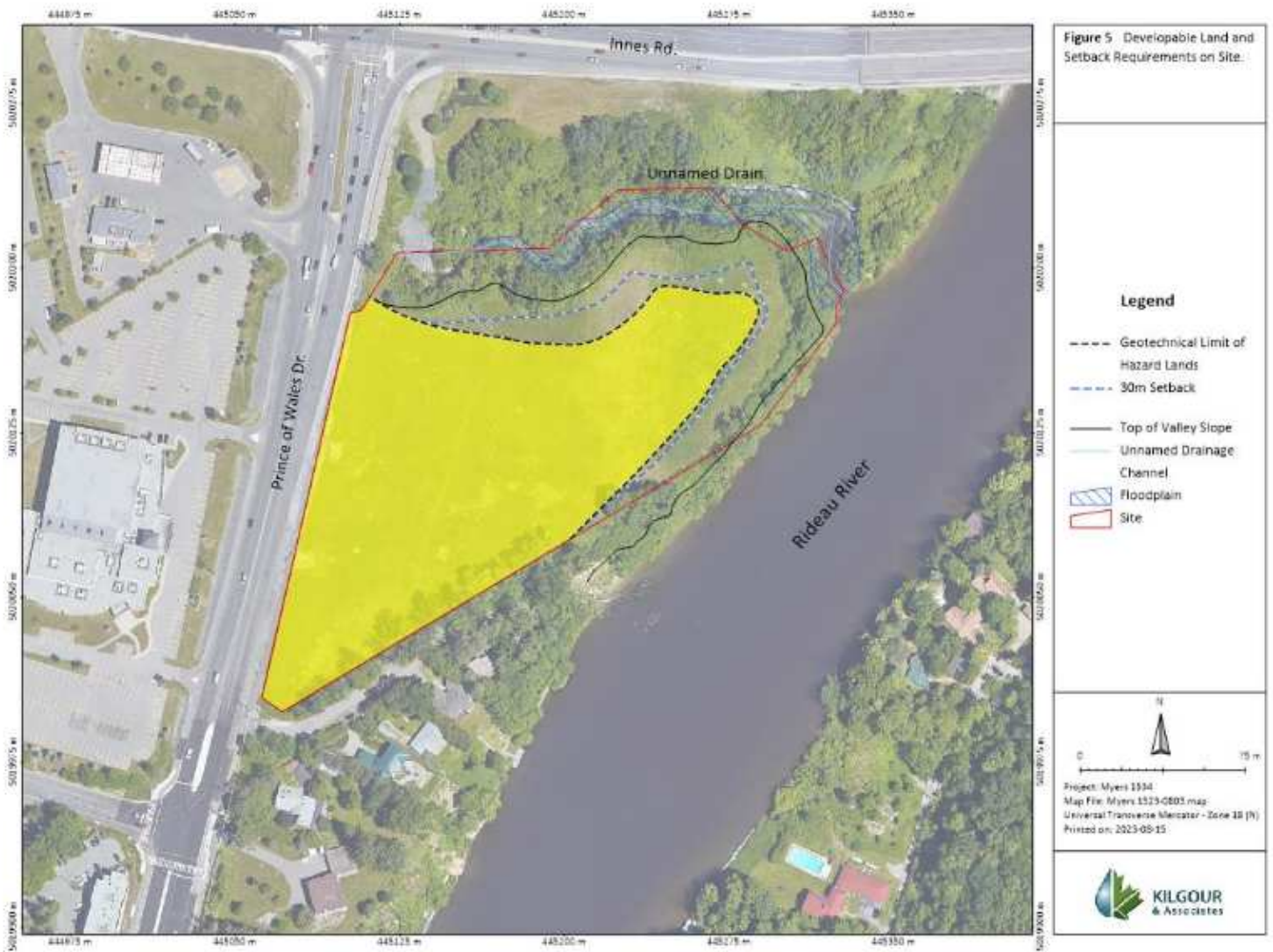
Figure 5 Developable Land and Setback Requirements on Site
