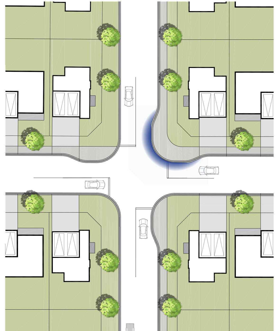
Figure 31 Double Bulb-Out at Intersection
