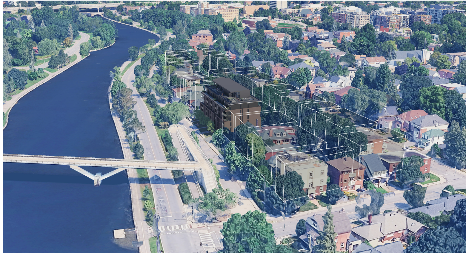
Aerial View of Site Looking North; Massing as per R4UD Zoning (14.5m building height)
