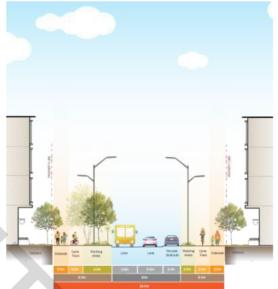
Figure 19: The Arch Conceptual Cross Section. Source: Fotenn
