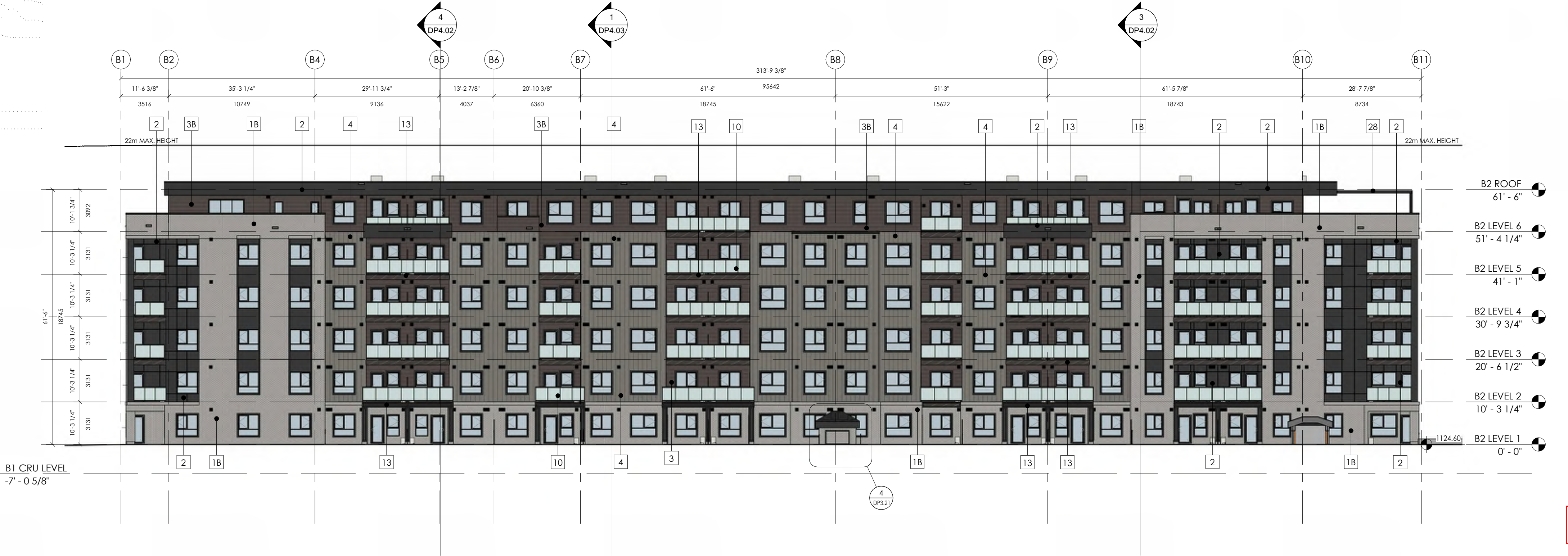
1 DP3.21 B2000 - EAST ELEVATION 1 : 200
