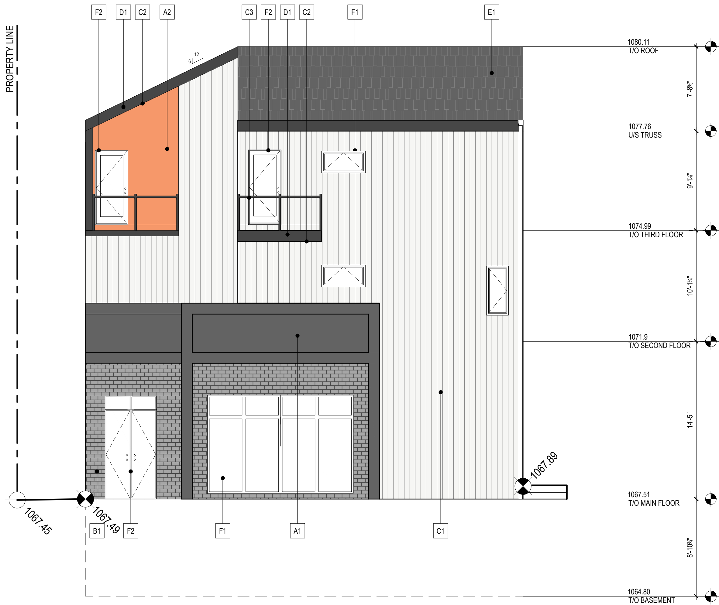
1 BUILDING A WEST ELEVATION DP.400 SCALE: 3/16" = 1'-0"
