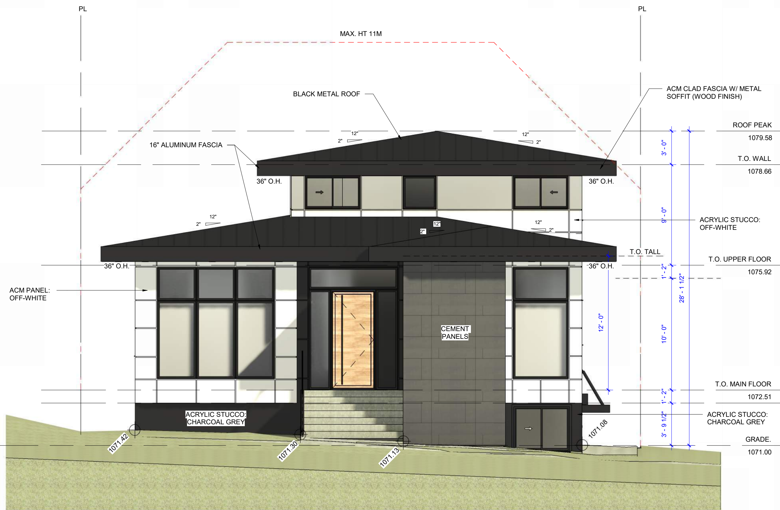
1 FRONT ELEVATION A3.0 3/16" = 1'-0"
