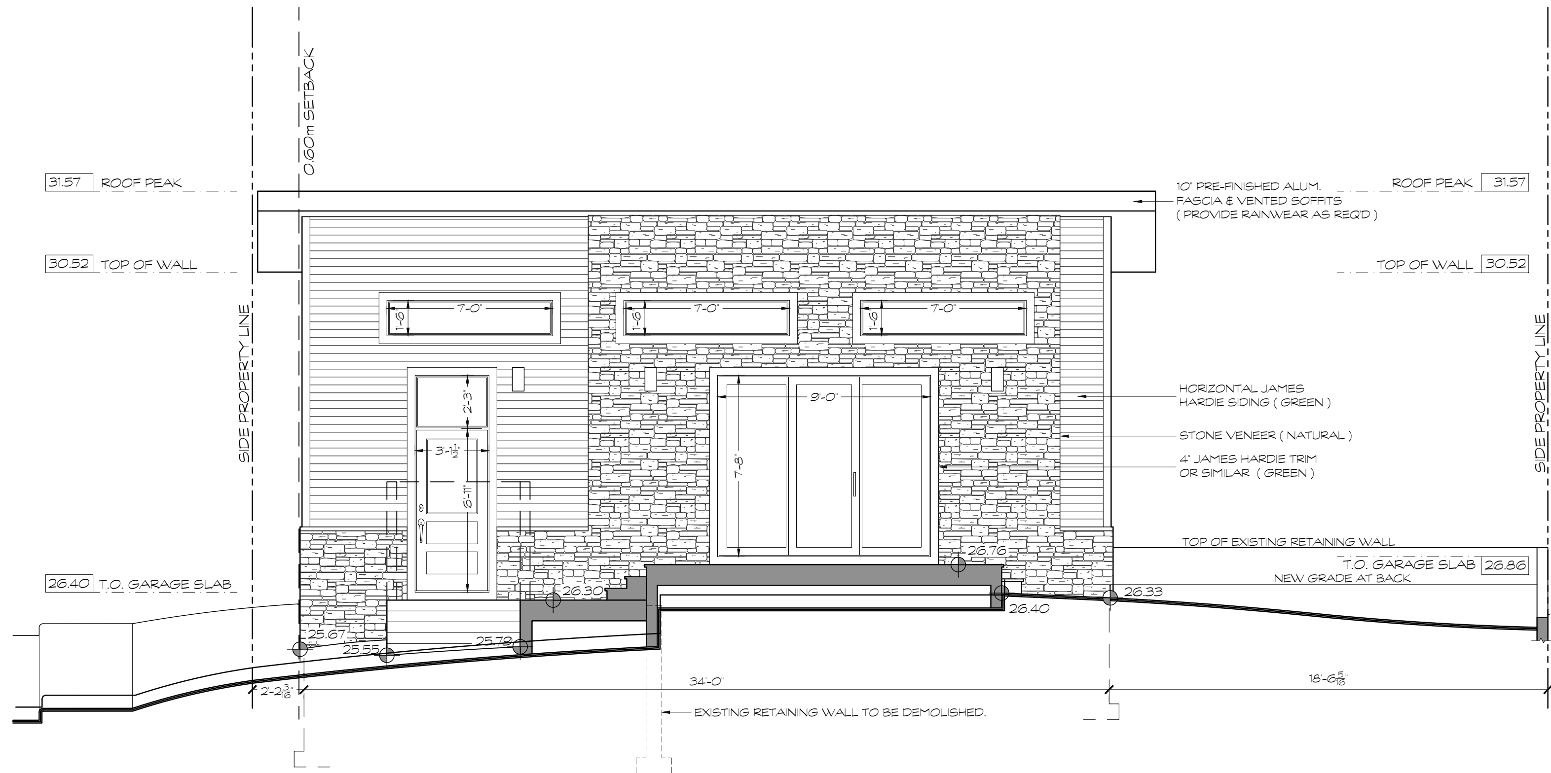
1 SOUTHWEST GARAGE ELEVATION A4 1/4" = 1'-0"
