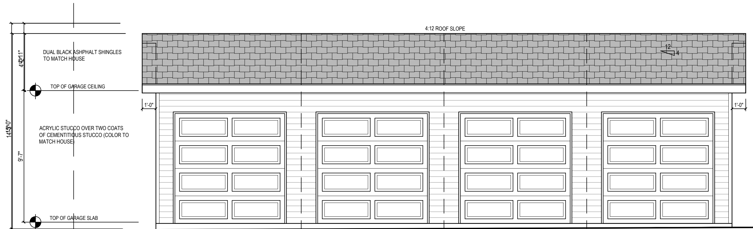
EAST ELEVATION SCALE: 1/4" = 1'-0"
