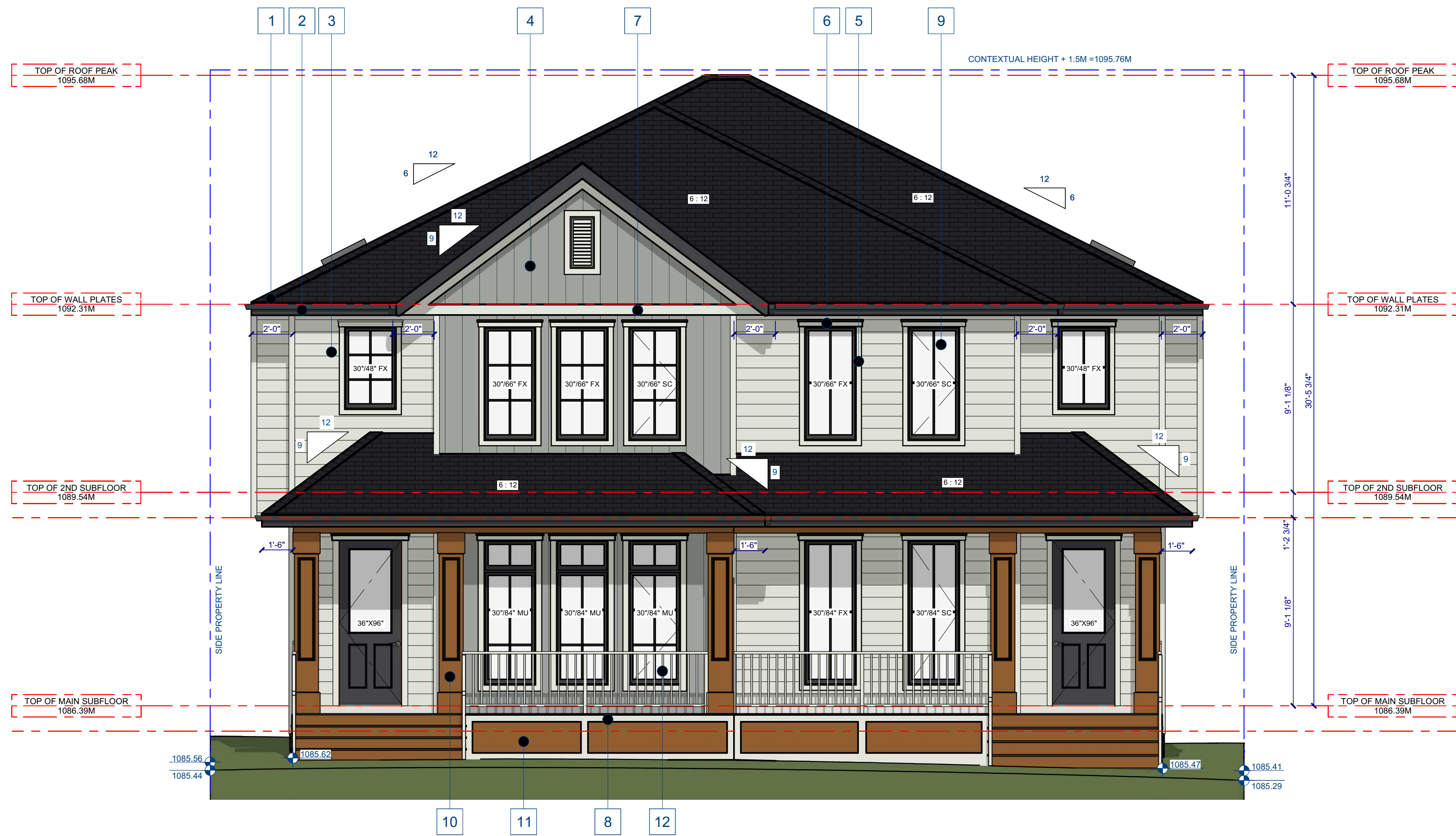
1 A5 FRONT ELEVATION SCALE = 1/4" = 1'-0"
