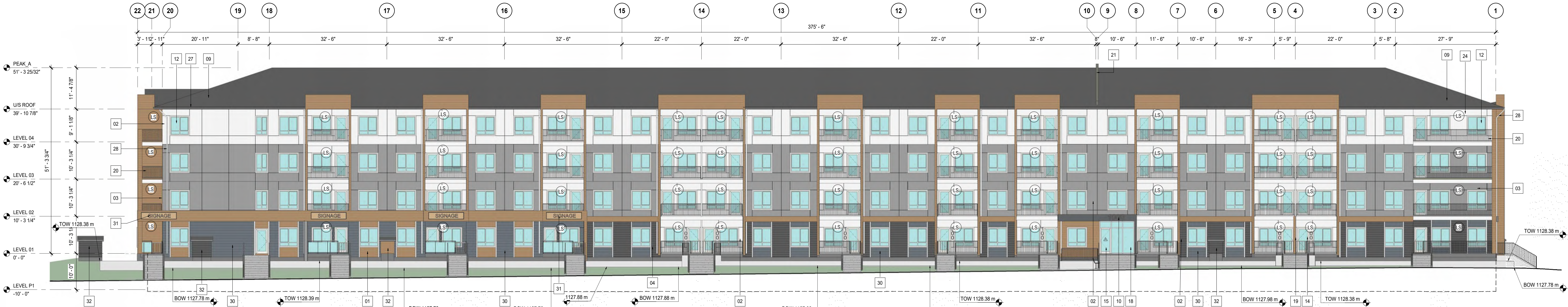
3 BUILDING A - EAST ELEVATION SCALE: 3/32" = 1'-0"
