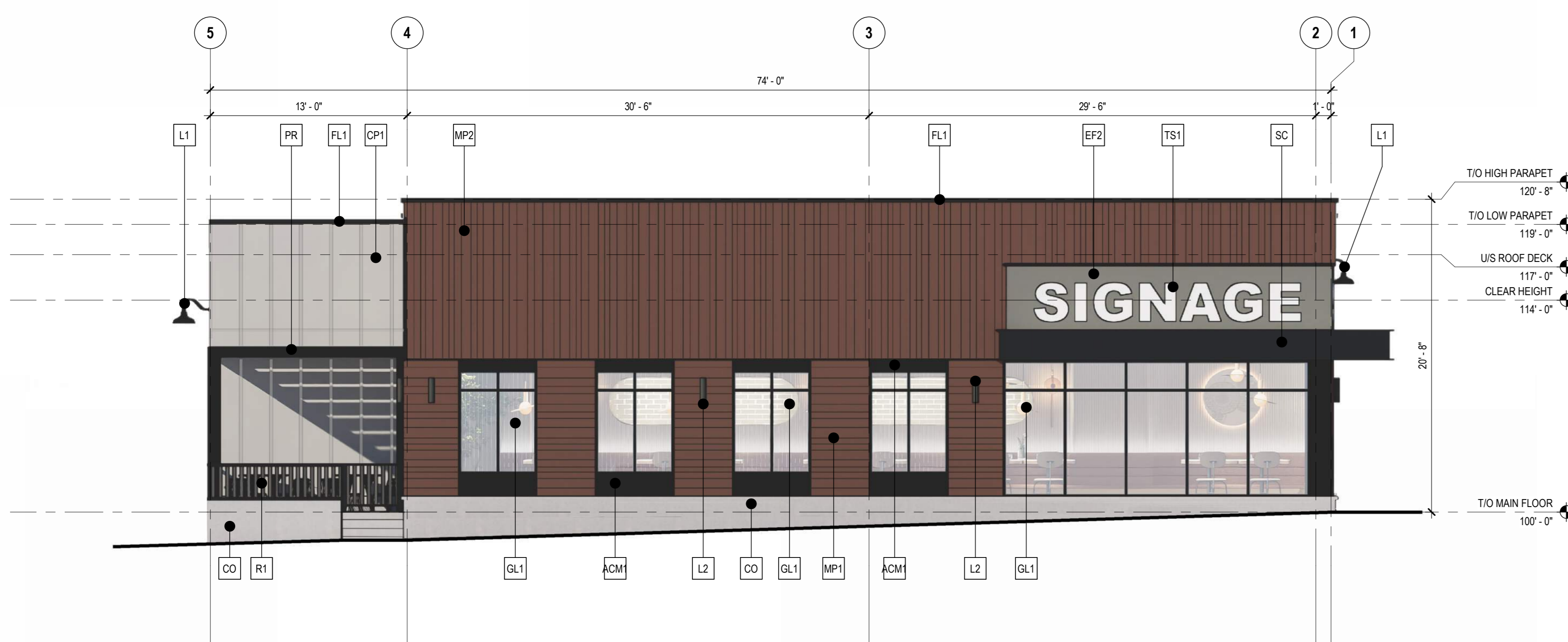
1 BUILDING 3 - NORTH ELEVATION SCALE: 3/16" = 1'-0"
