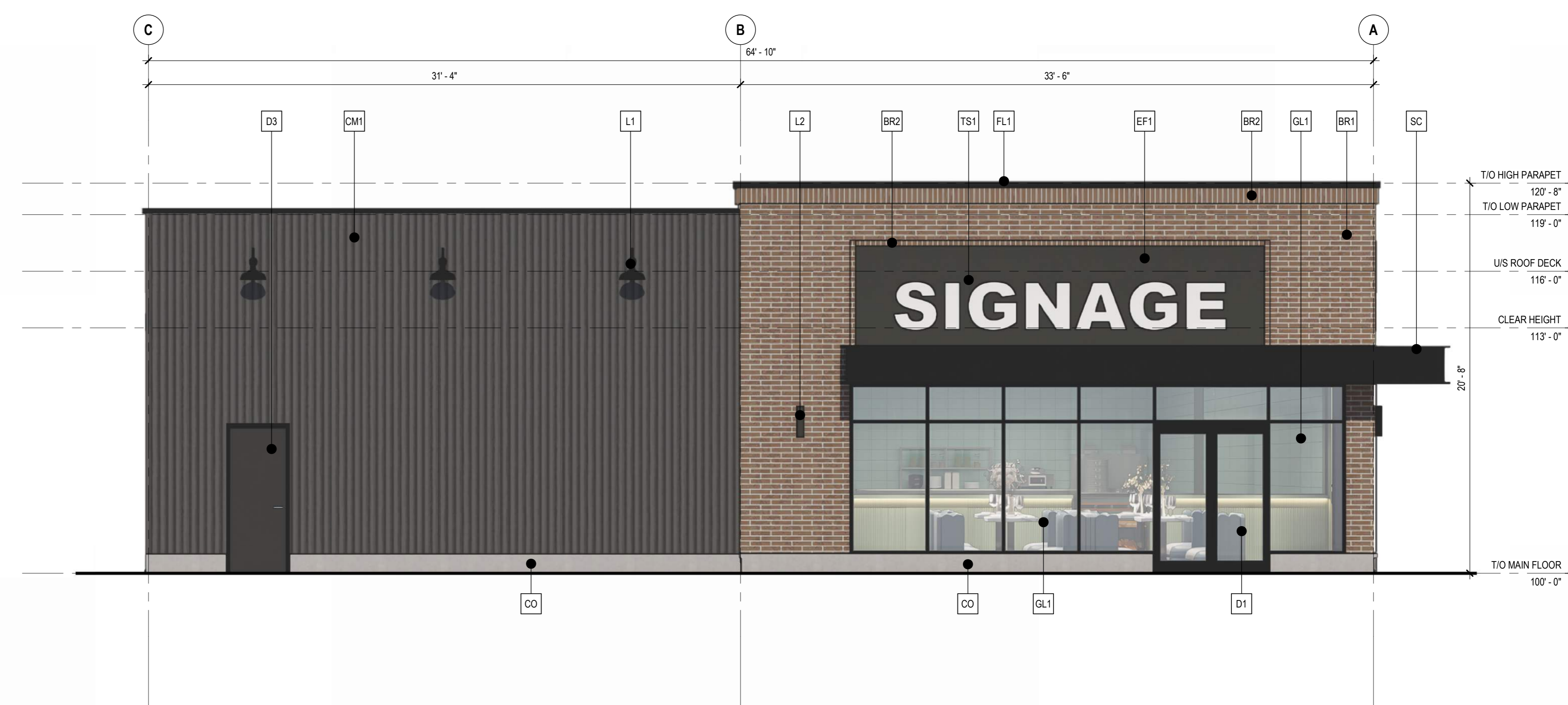
2 BUILDING 1 - EAST ELEVATION SCALE: 1/4" = 1'-0"
