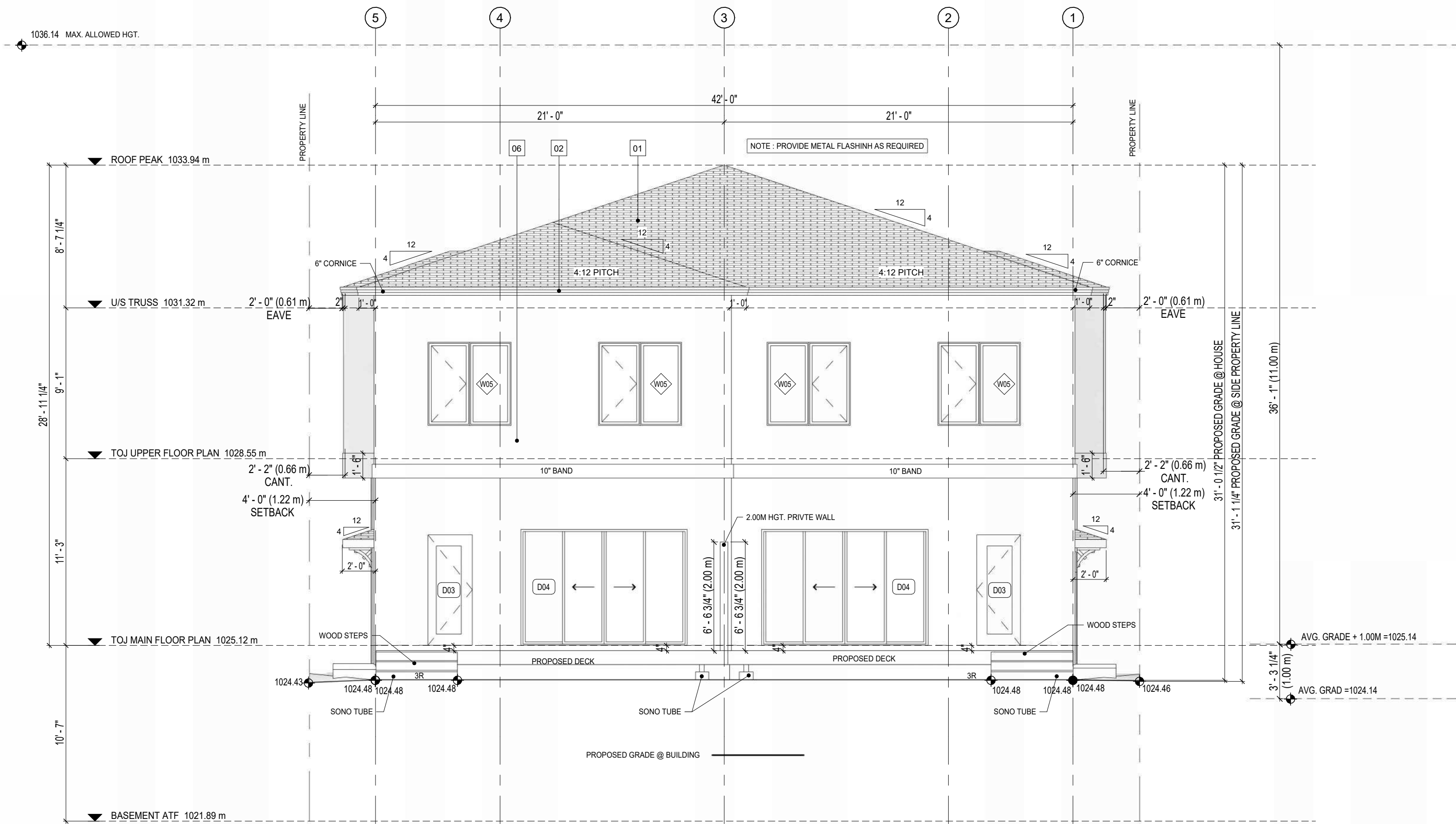
2 PROPOSED REAR (WEST) ELEVATION 3/16" = 1'-0"
