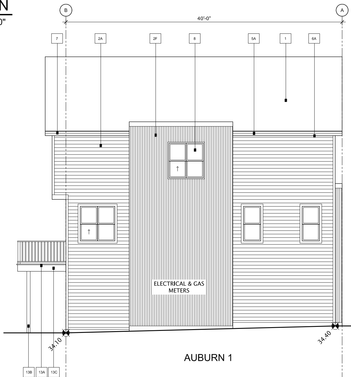
3 BUILDING 14 EAST ELEVATION SCALE 1/8" = 1'- 0"
