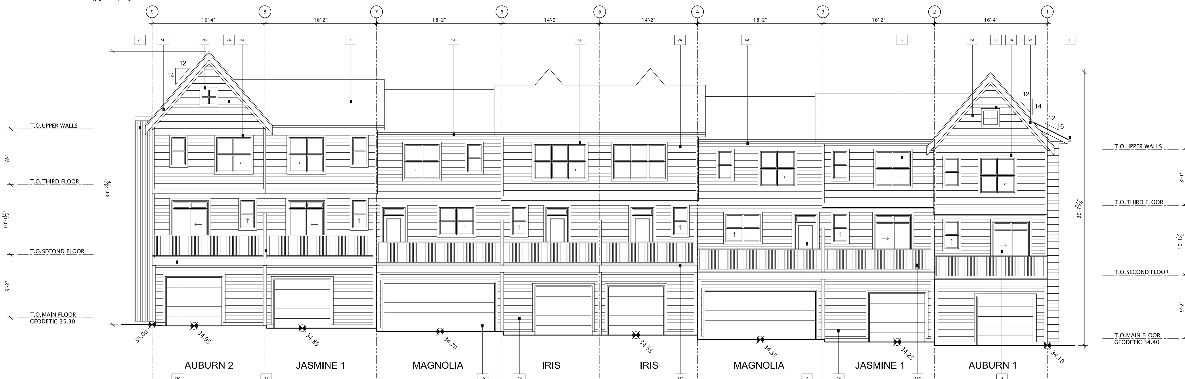
2 BUILDING 8 NORTH ELEVATION SCALE 1/8" = 1'-0"
