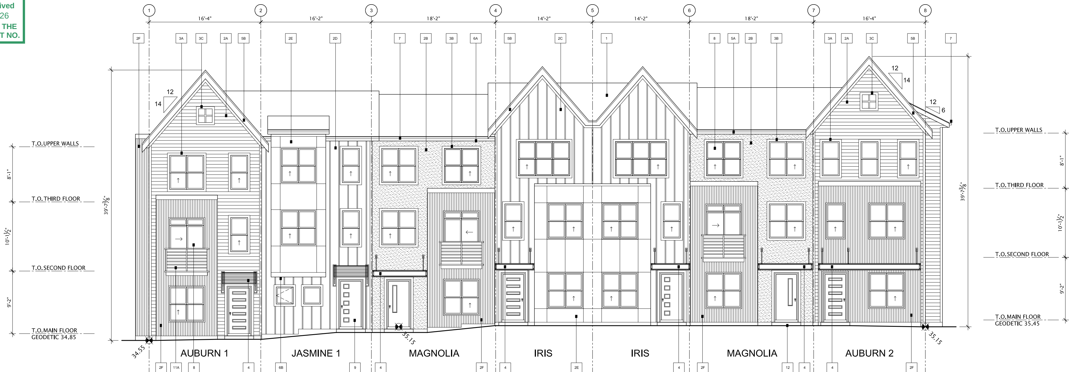
1 BUILDING 13 EAST ELEVATION SCALE 1/8" = 1'-0"
