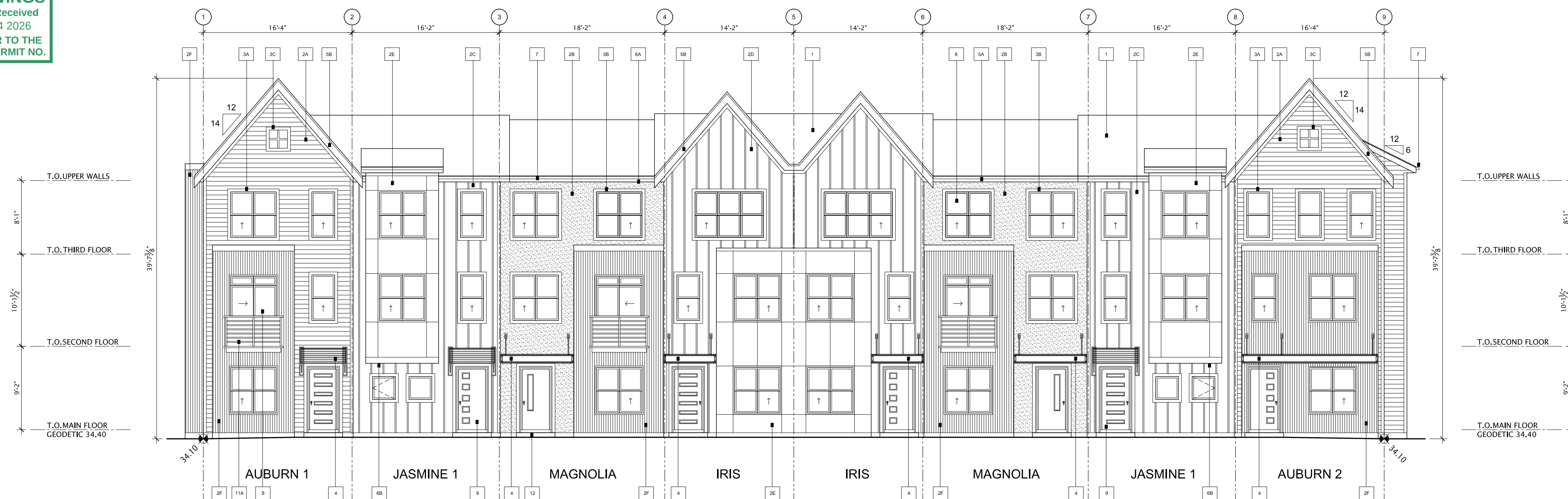
1 BUILDING 7 SOUTH ELEVATION SCALE 1/8" = 1'-0"
