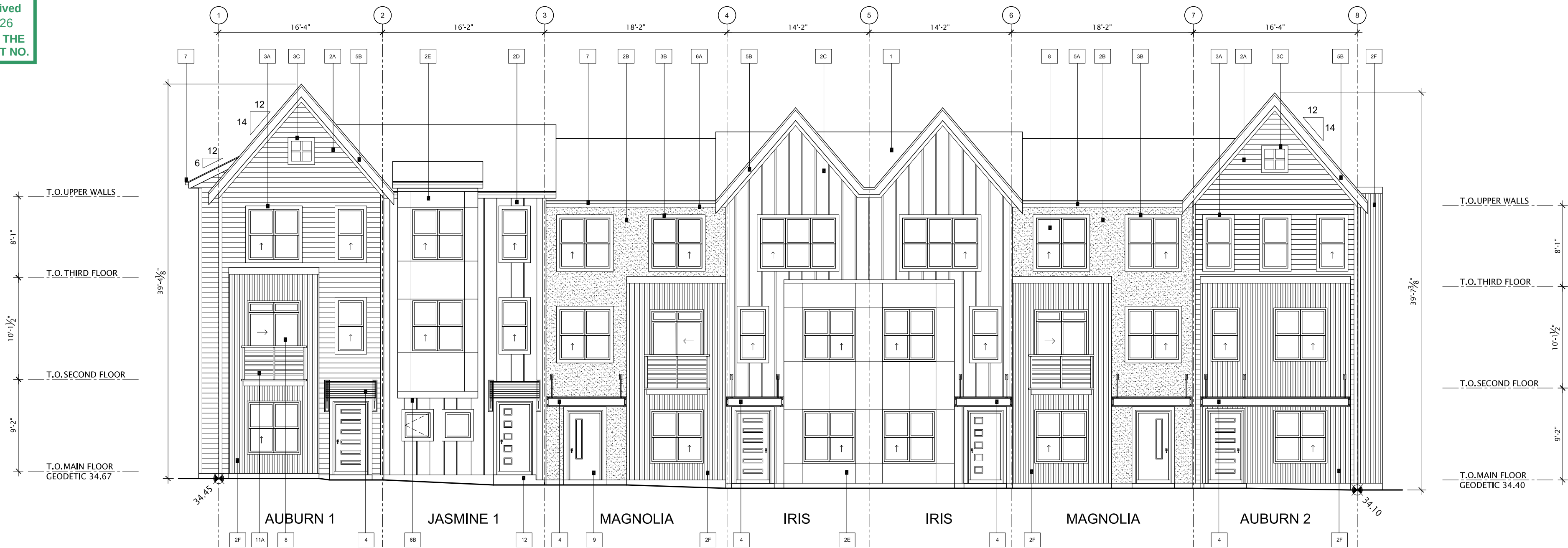
1 BUILDING 6 WEST ELEVATION SCALE 1/8" = 1'-0"
