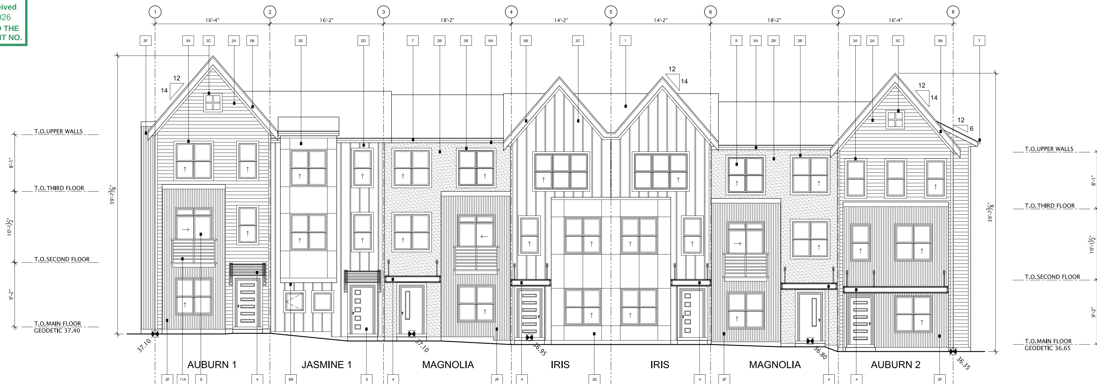
1 BUILDING 3 WEST ELEVATION SCALE 1/8" = 1' - 0"
