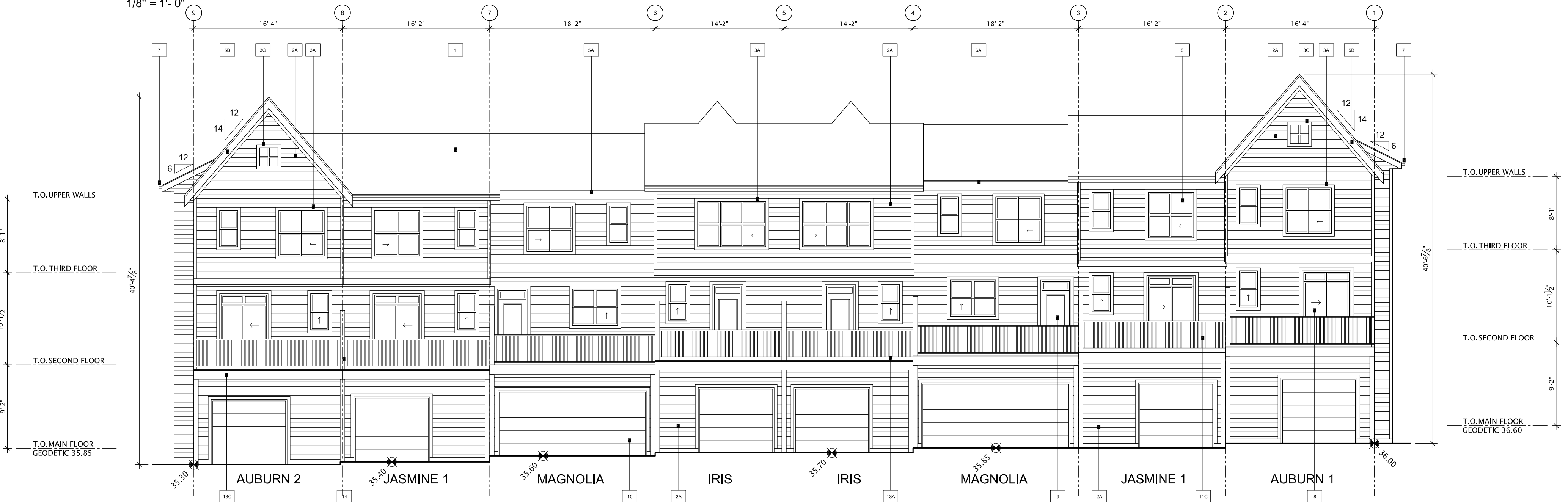
2 BUILDING 4 EAST ELEVATION SCALE 1/8" = 1'-0"
