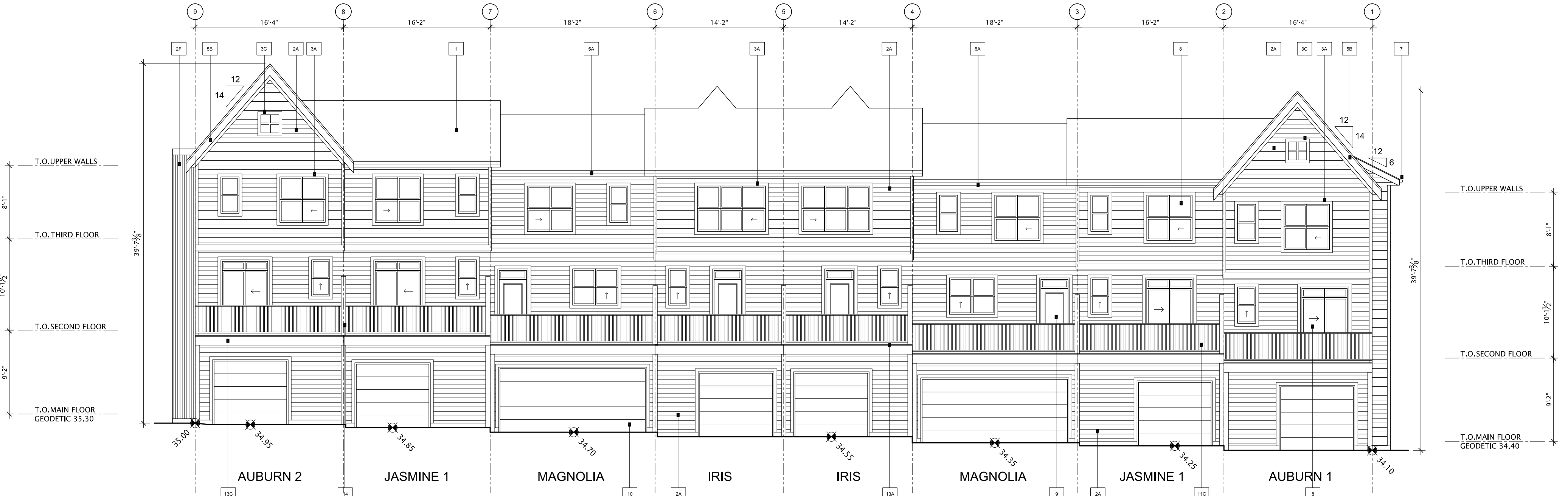
2 BUILDING 8 NORTH ELEVATION SCALE 1/8" = 1'-0"
