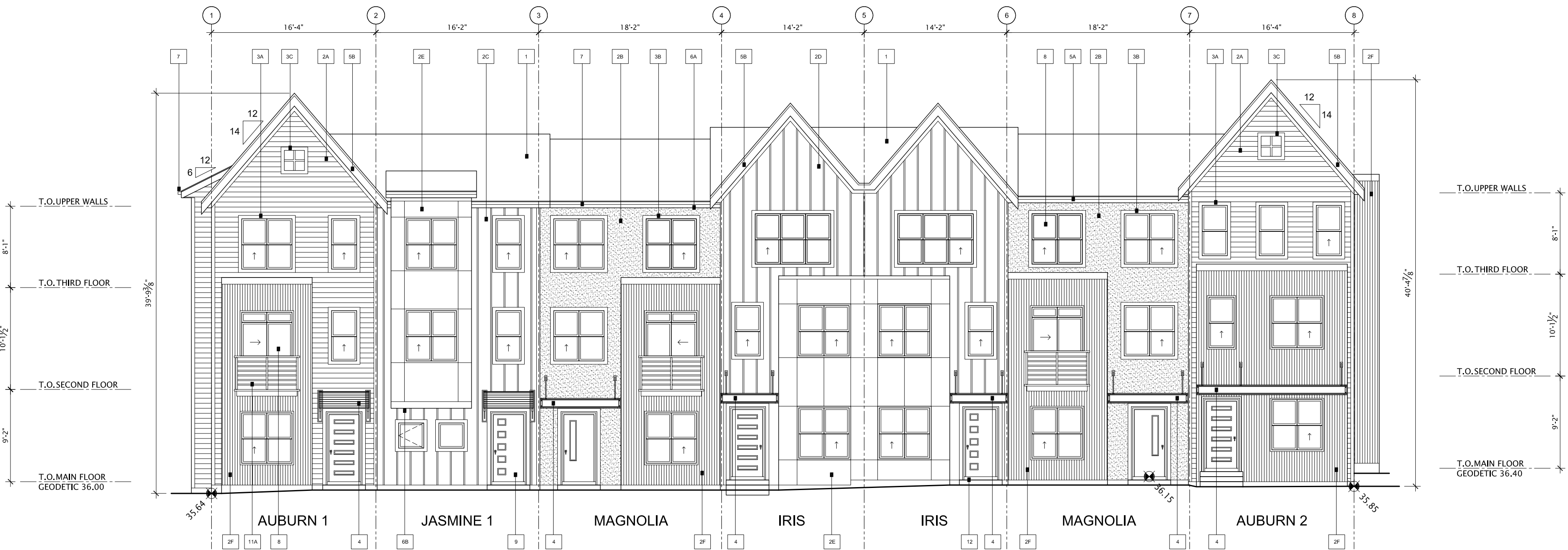
1 BUILDING 12 EAST ELEVATION SCALE 1/8" = 1'-0"
