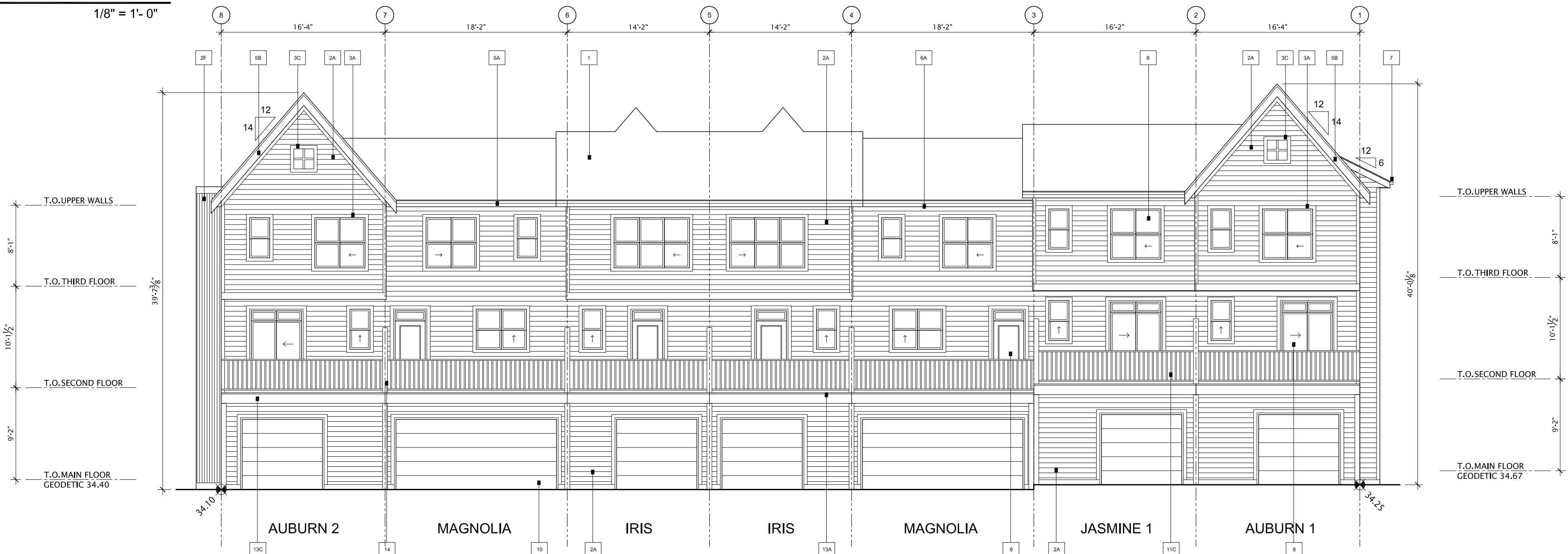
2 BUILDING 6 EAST ELEVATION SCALE 1/8" = 1'-0"
