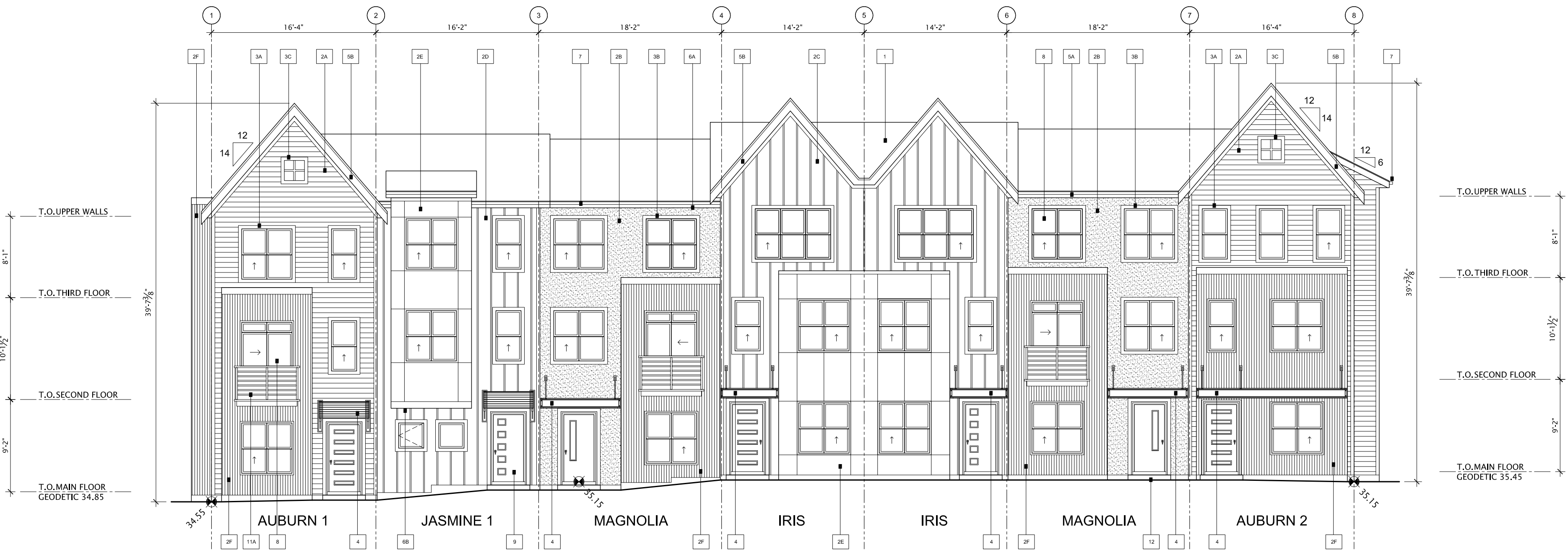
1 BUILDING 13 EAST ELEVATION SCALE 1/8" = 1'-0"
