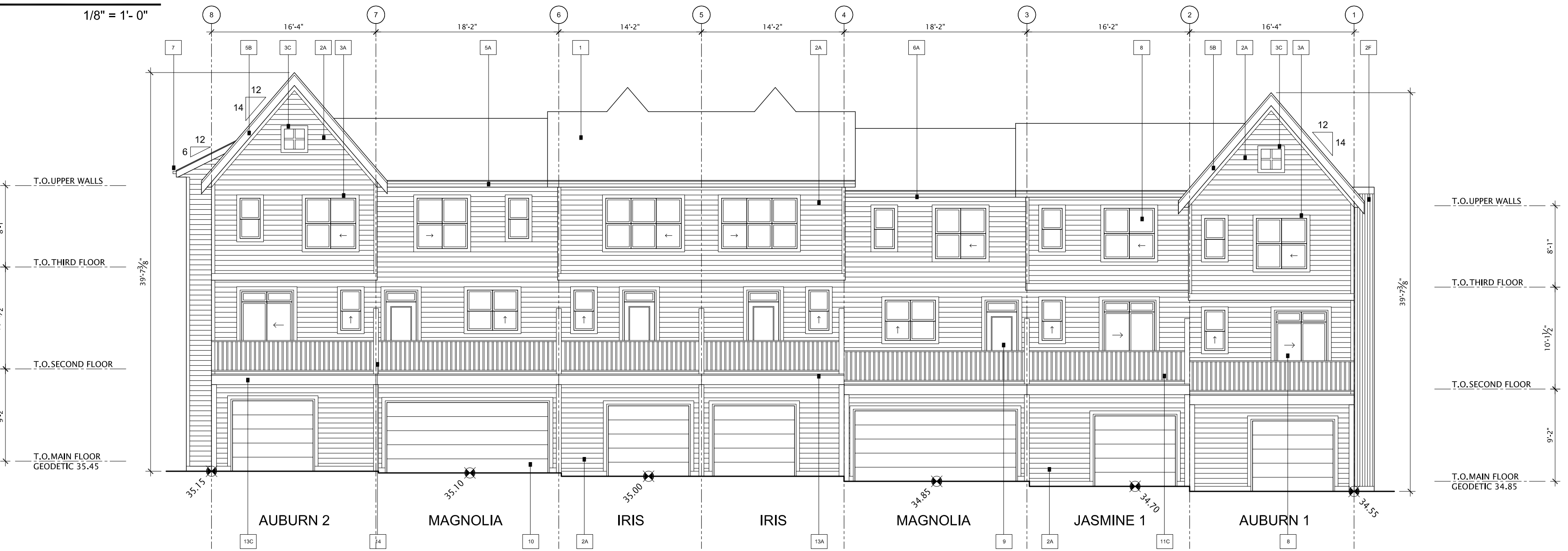
2 BUILDING 13 WEST ELEVATION SCALE 1/8" = 1'-0"
