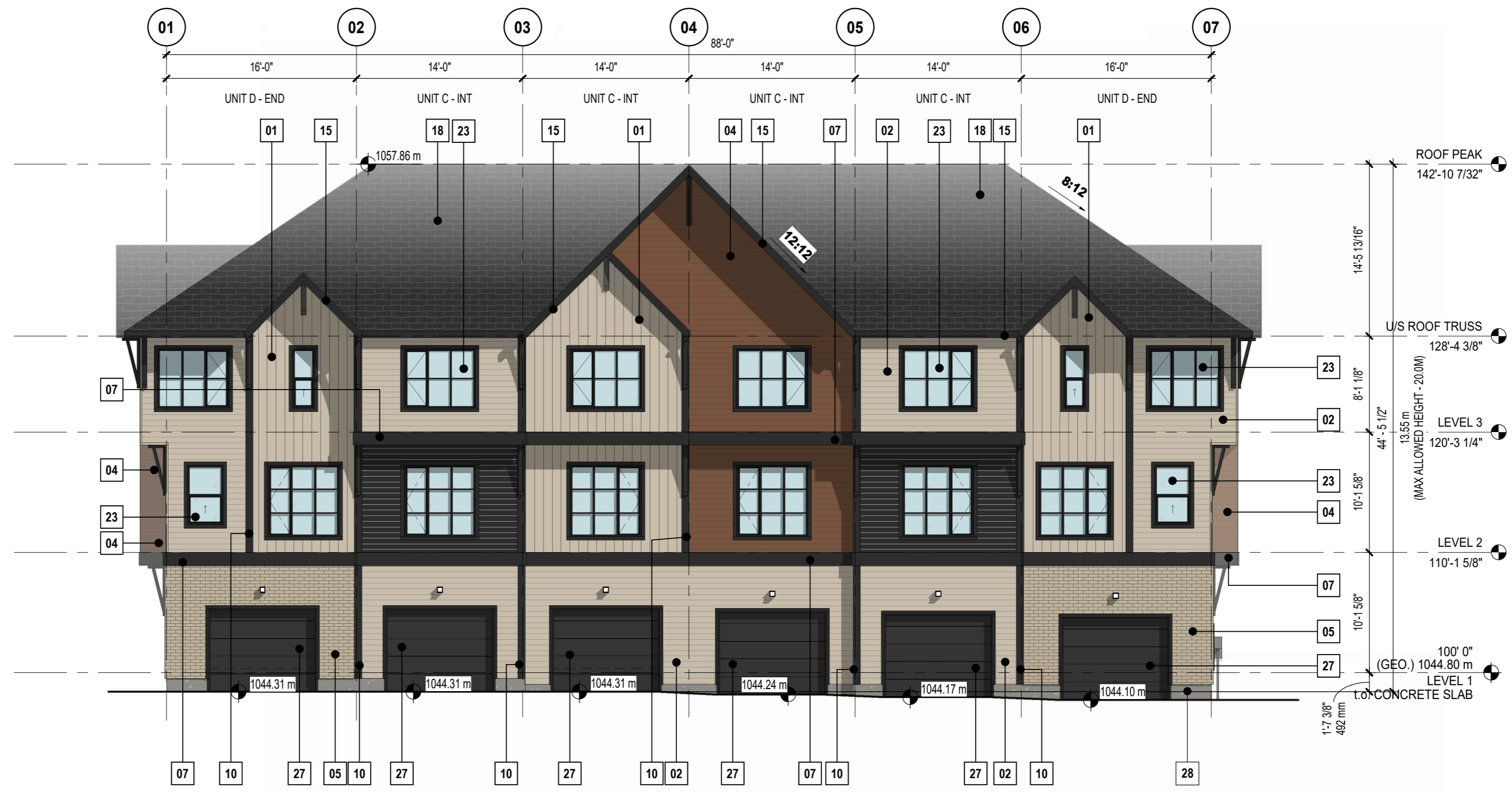
2 BUILDING 04 - NORTH-WEST ELEVATION DP40-04-01 SCALE: 1/8" = 1'-0"
