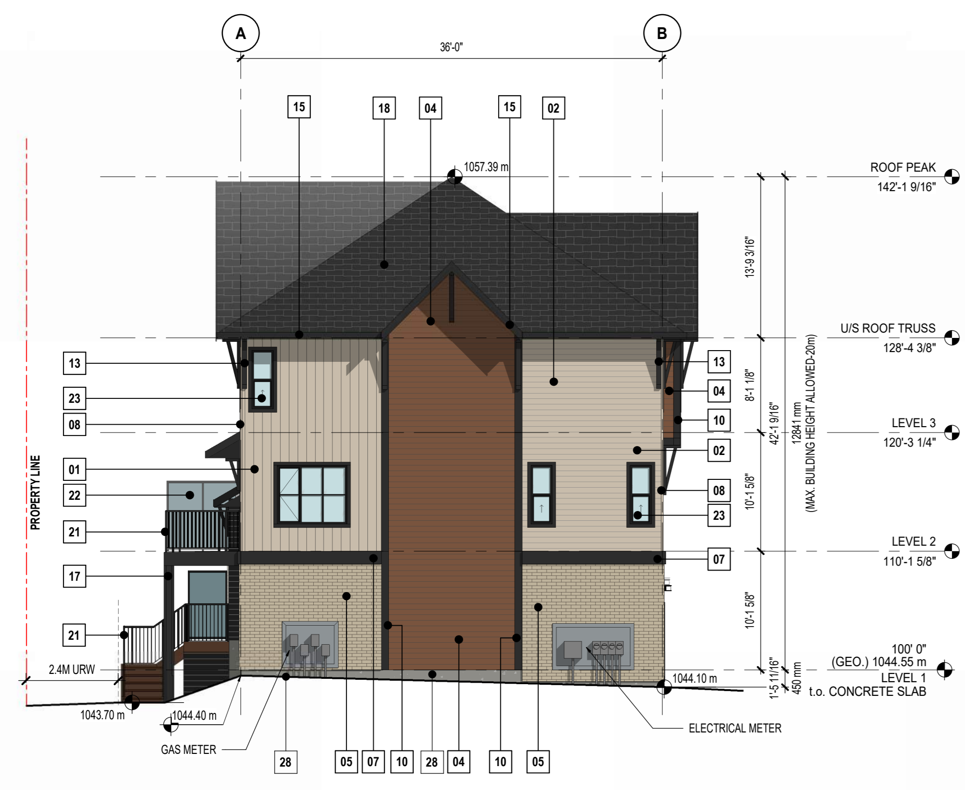
3 BUILDING 03 - SOUTH-WEST ELEVATION DP40-03-01 SCALE: 1/8" = 1'-0"
