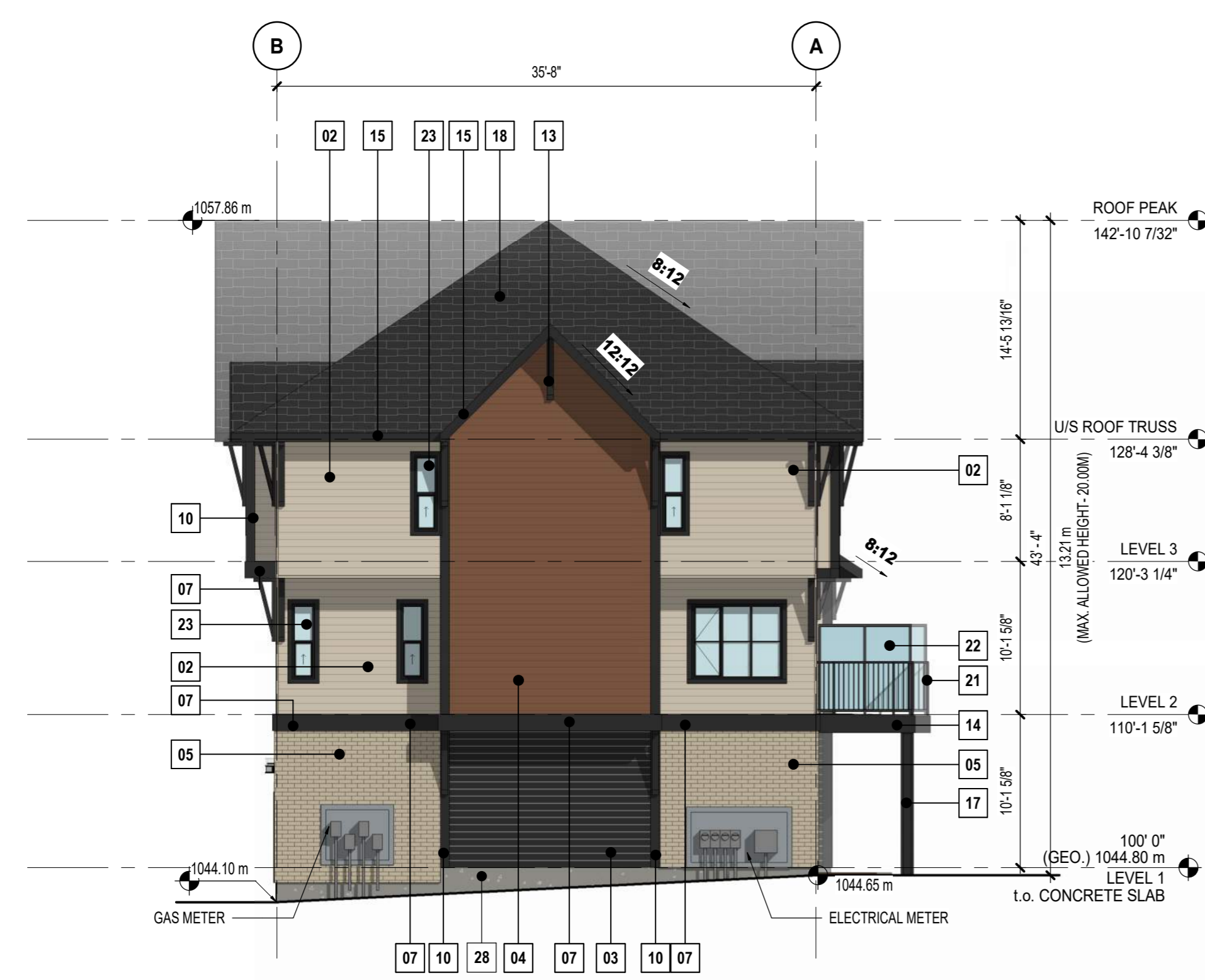
3 BUILDING 04 - SOUTH-WEST ELEVATION DP40-04-01 SCALE: 1/8" = 1'-0"
