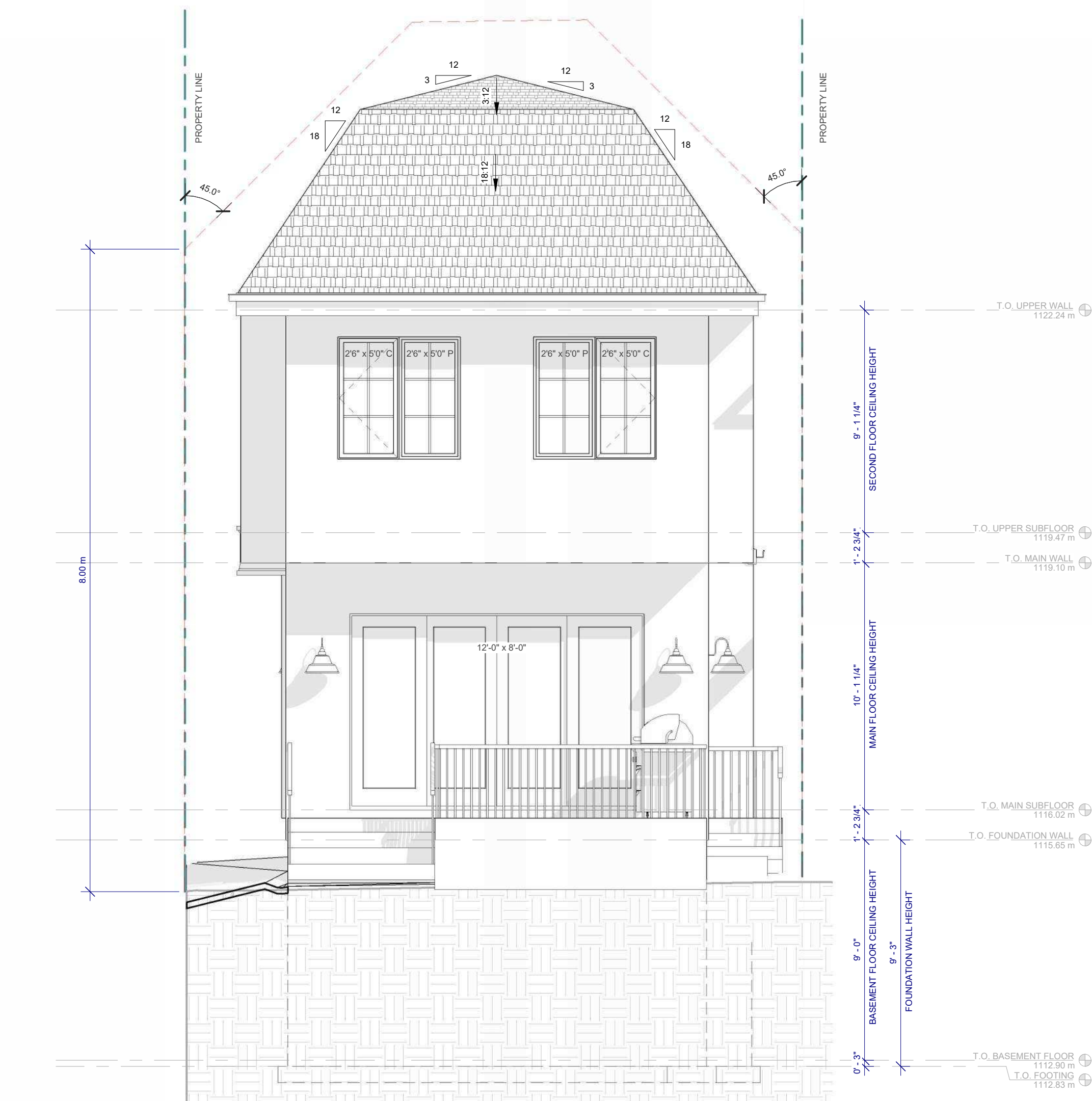
BUILDING 2 - REAR ELEVATION 1/4" = 1'-0"
