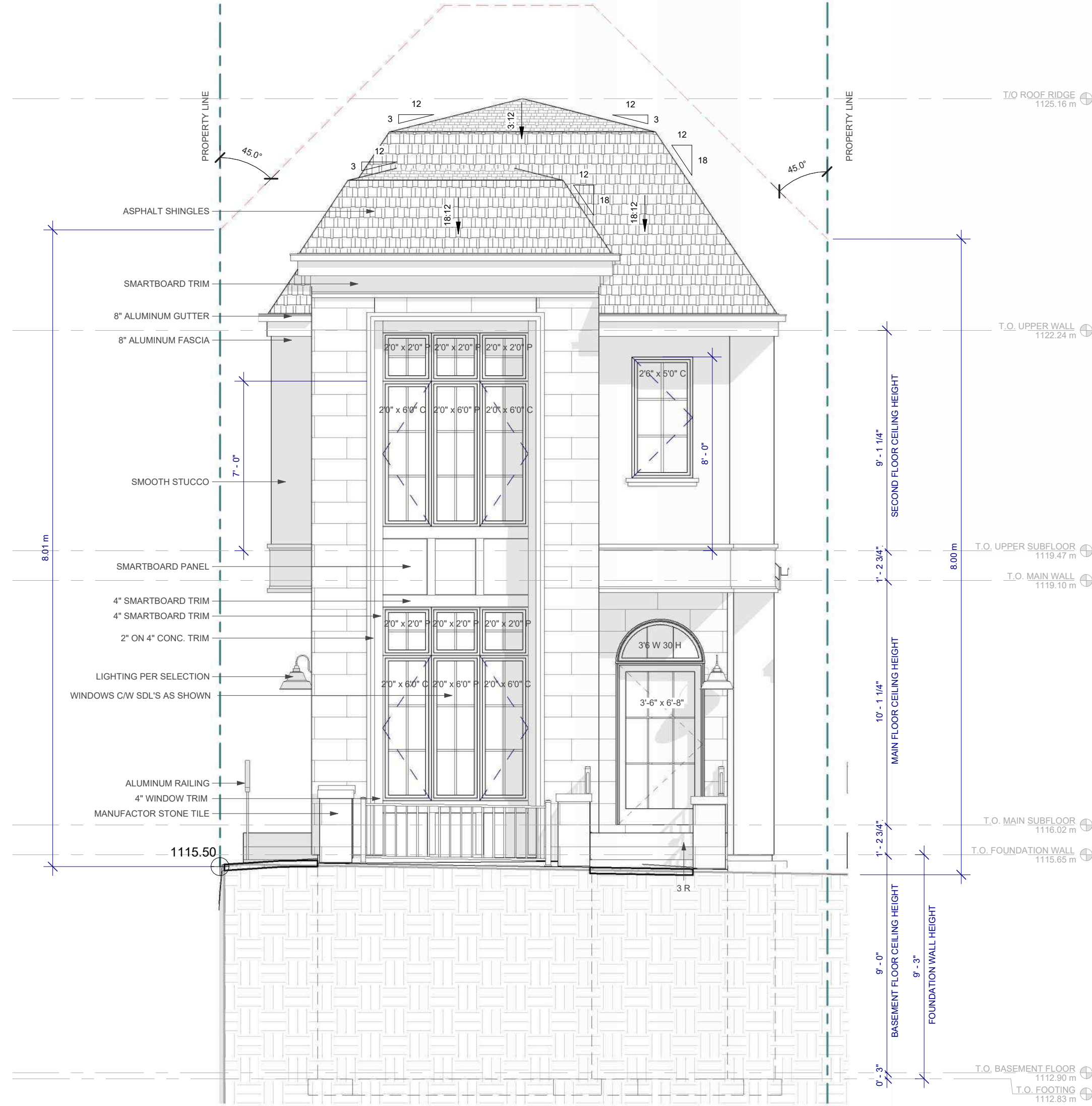
1 BLDG 1 - FRONT ELEVATION 1/4" = 1'-0"
