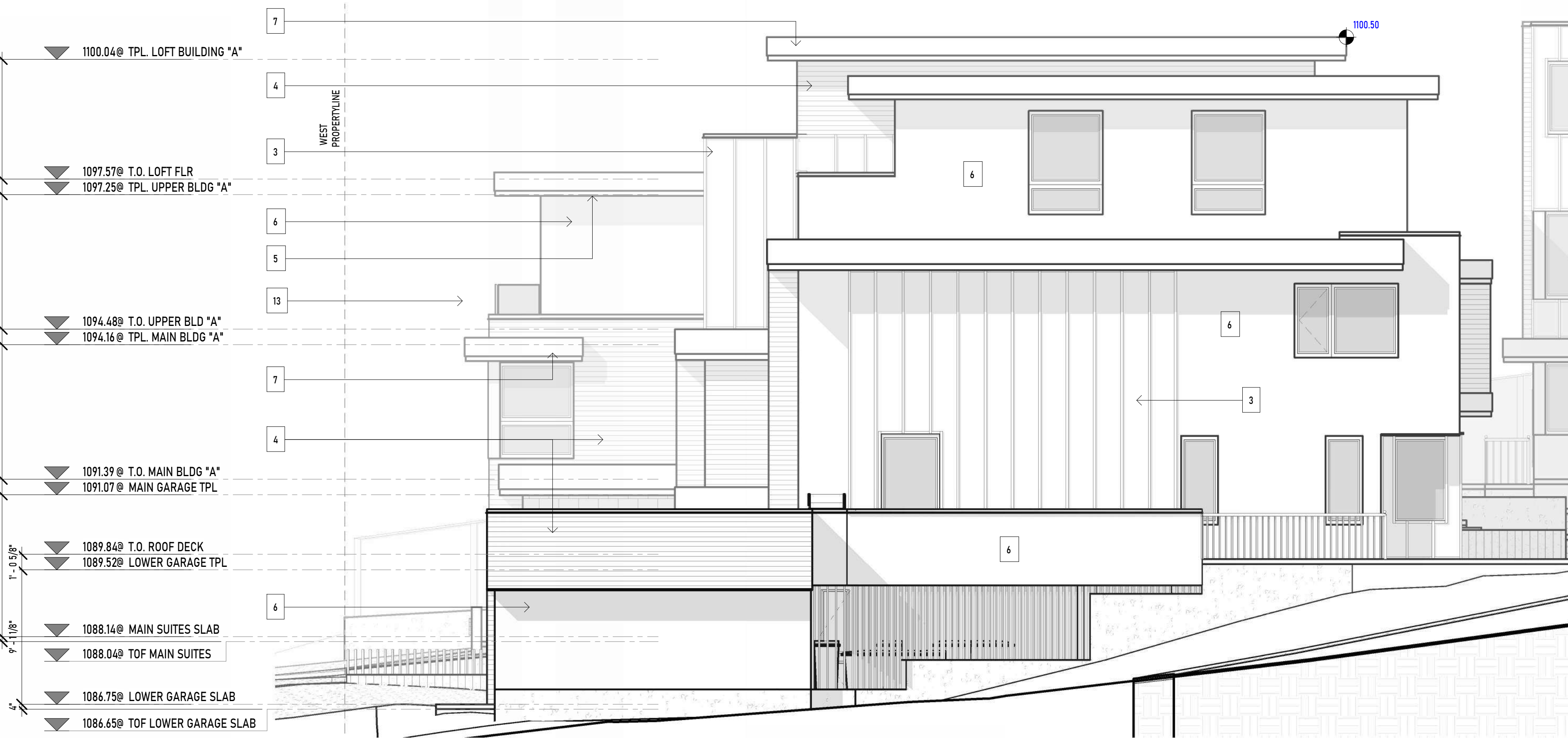
2 BUILDING "A" SOUTH ELEVATION
