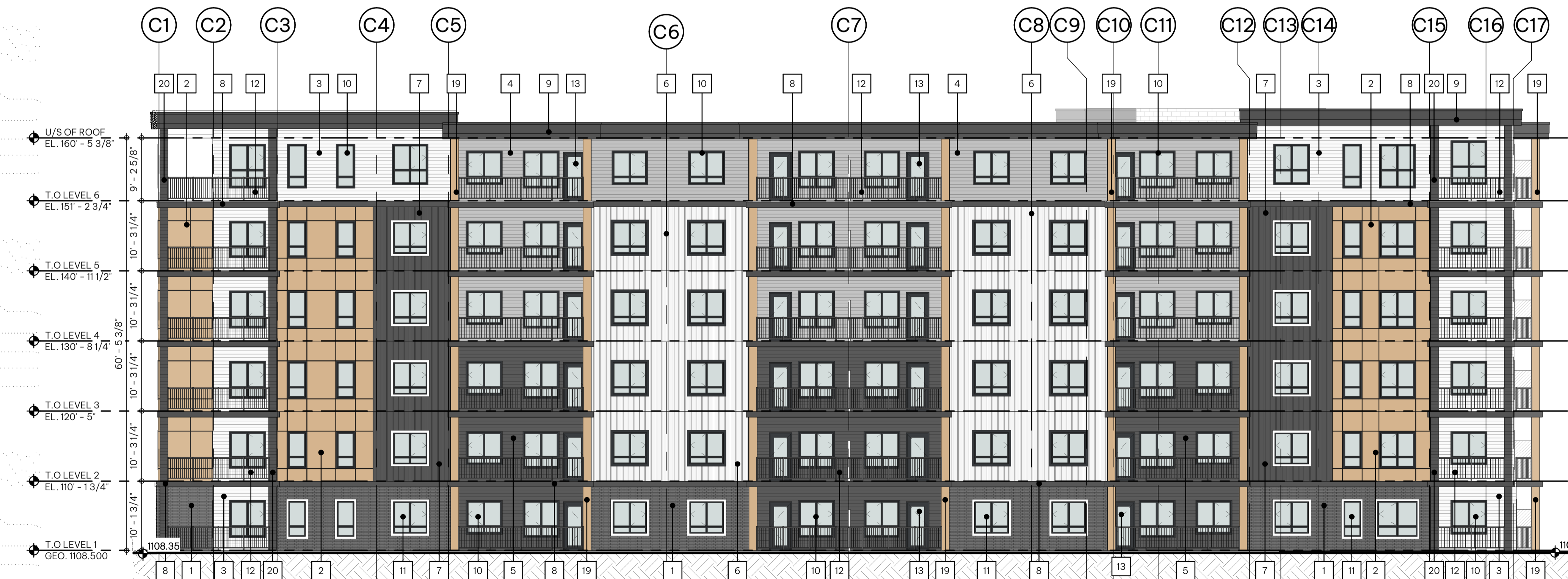
2 Building C - South Elevation 1 DP4.31 SCALE: 3/32" = 1'-0"
