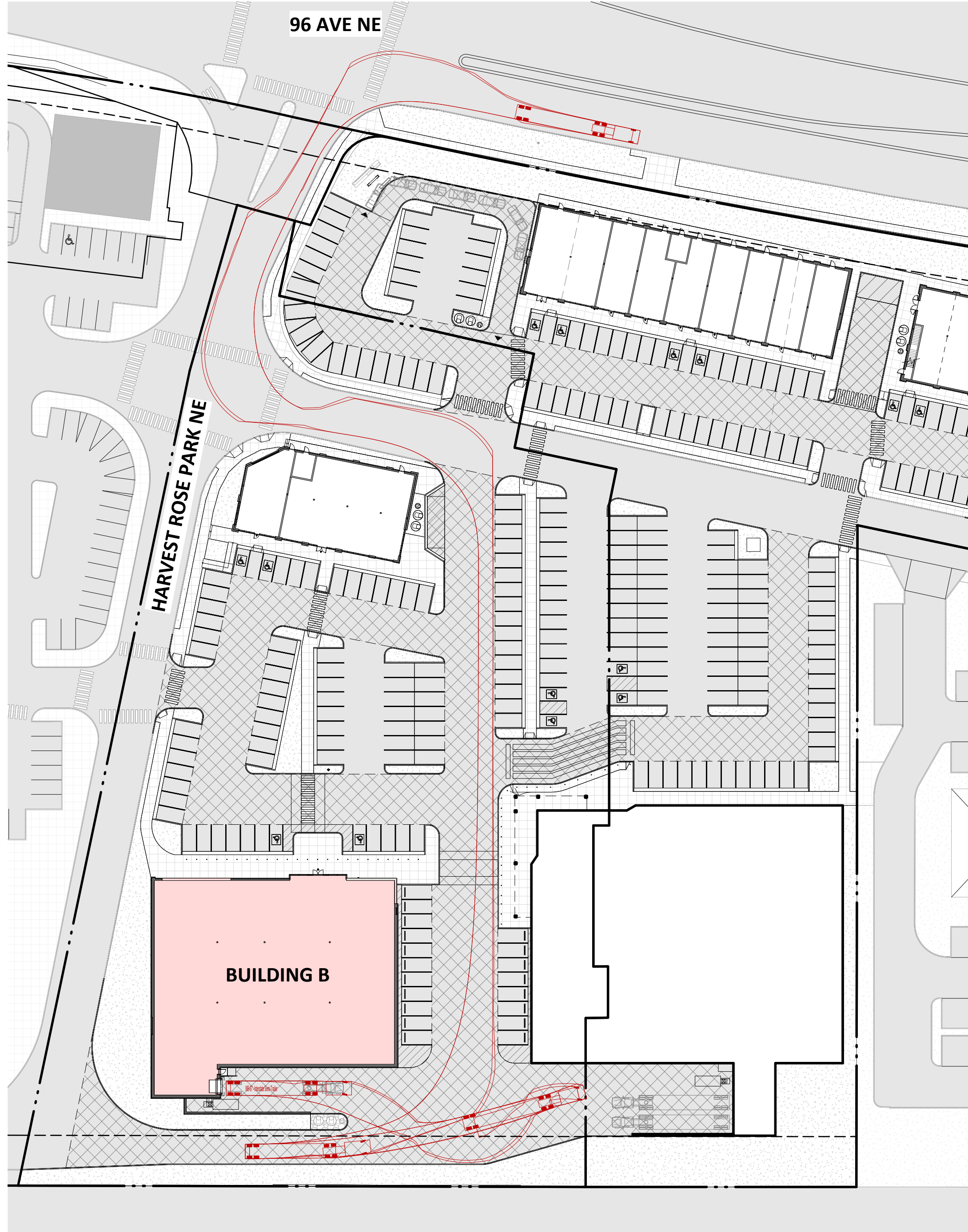
4 TRUCK MOVEMENT - BUILDING B OUT DP10.05 1:600 NORTH
