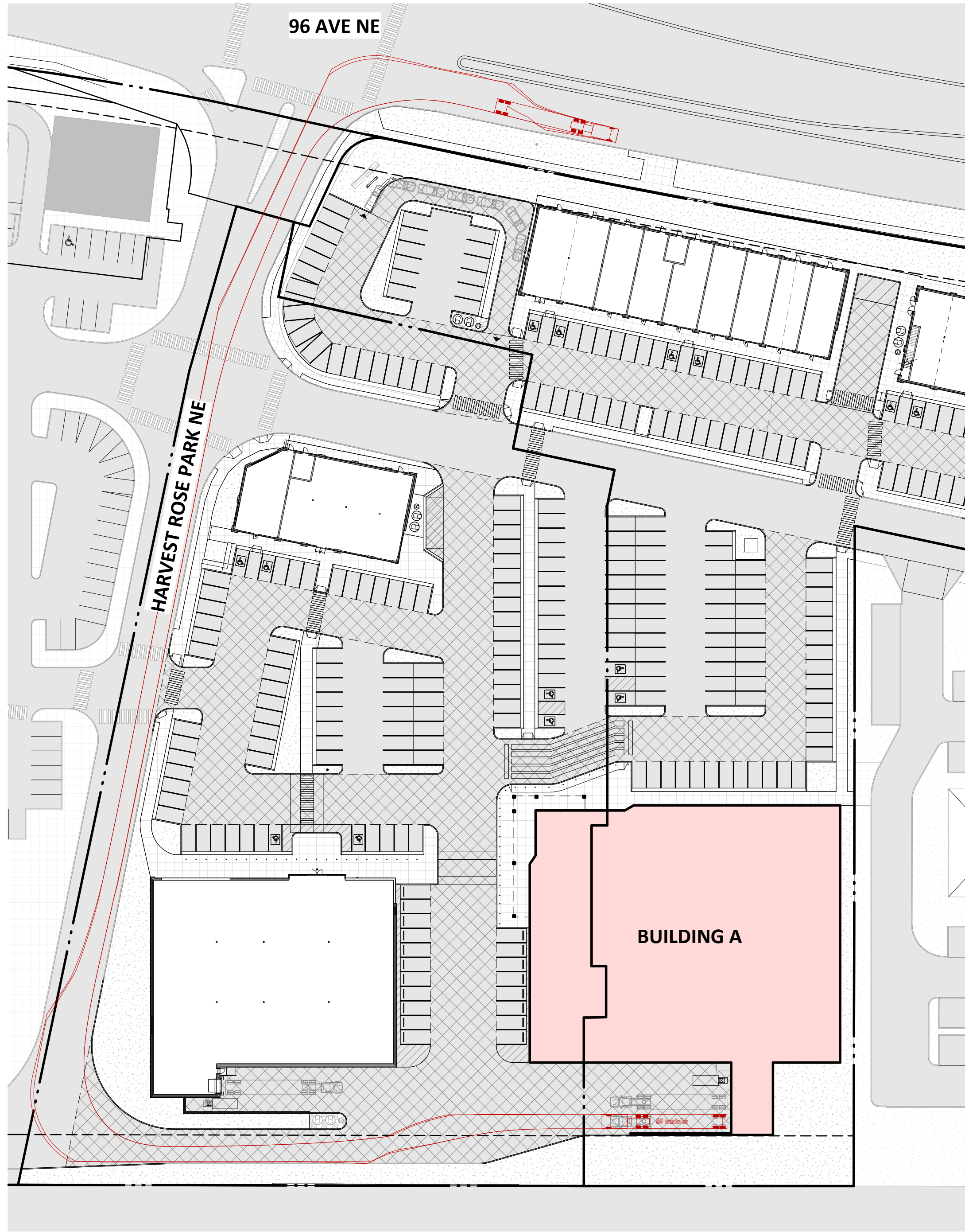
2 TRUCK MOVEMENT - BUILDING A OUT DP10.05 1:600 NORTH
