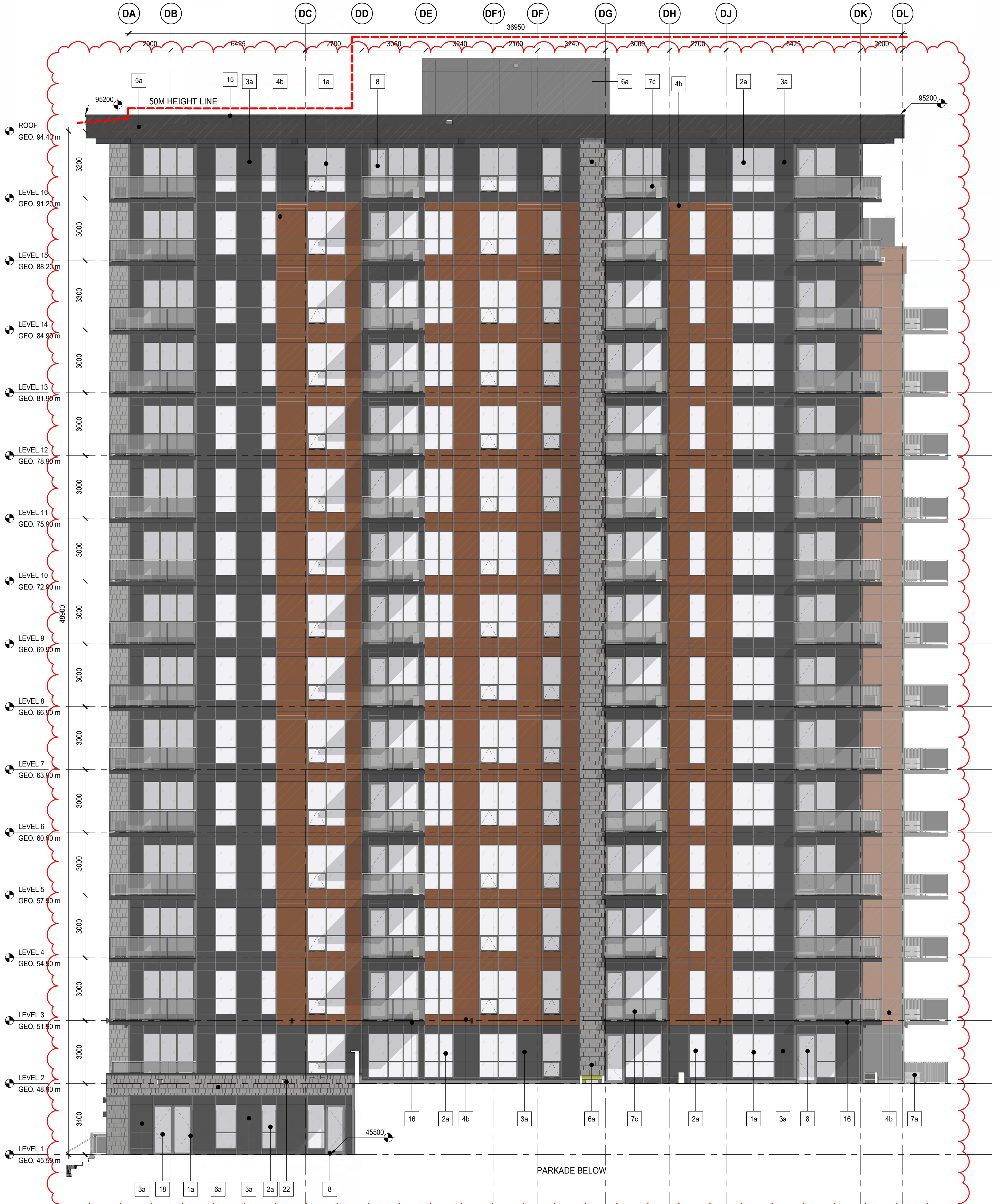
2 TOWER D - WEST ELEVATION DP40-05-01 SCALE: 1: 100
