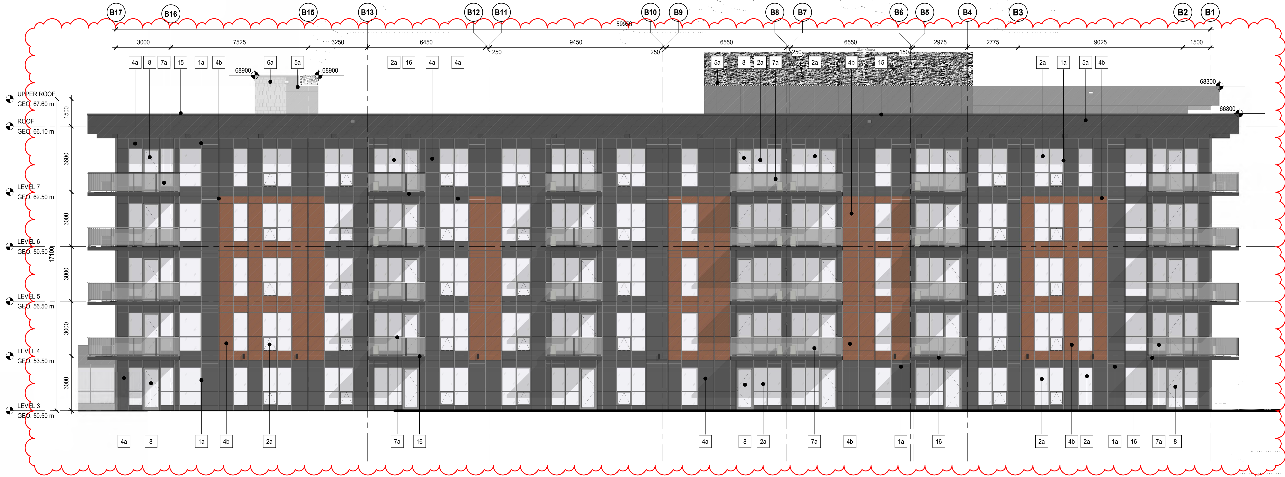
2 BUILDING B - WEST ELEVATION DP40-03-01 SCALE: 1:100
