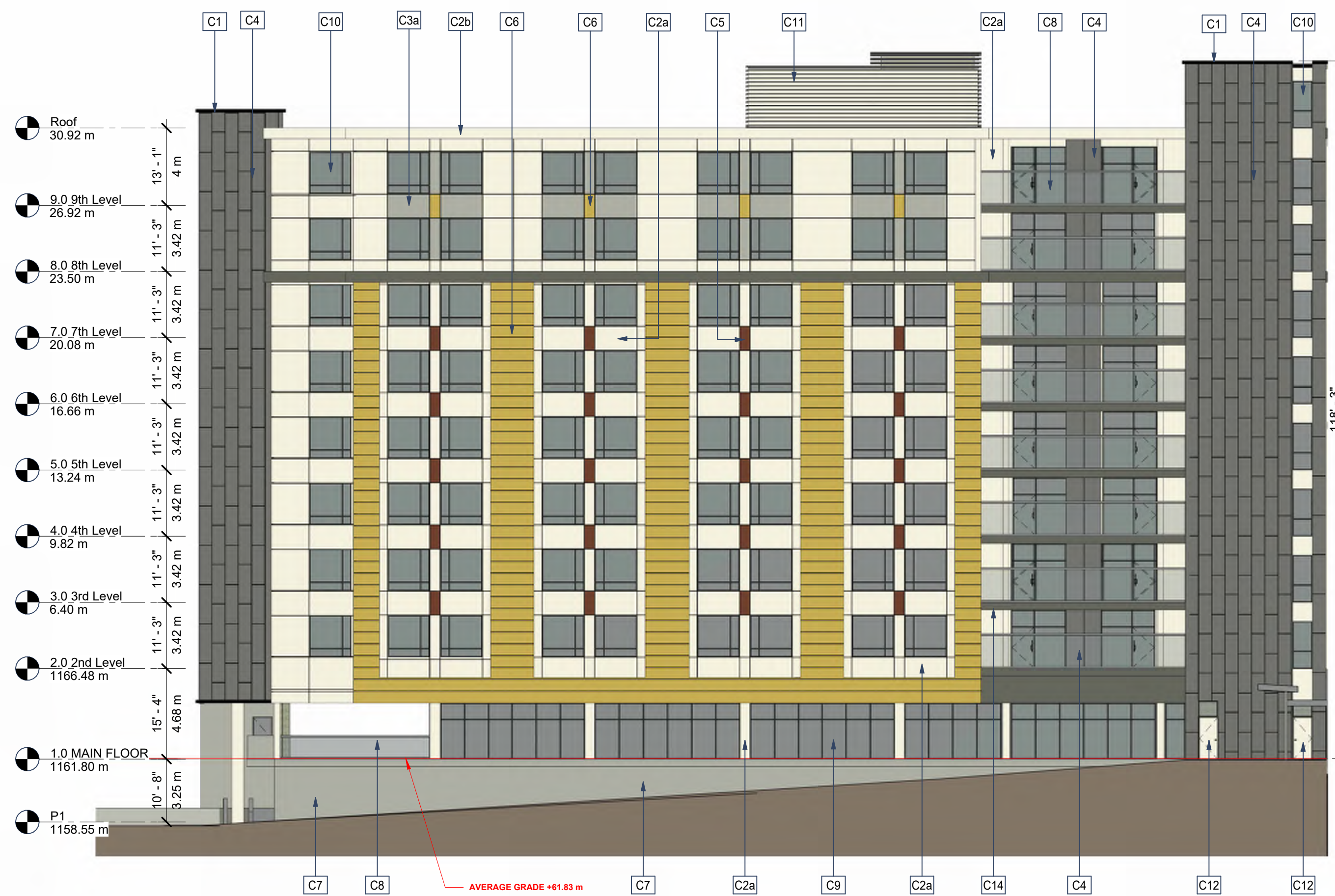
1 NORTH-EAST ELEVATION SCALE: 1/16" = 1'-0"
