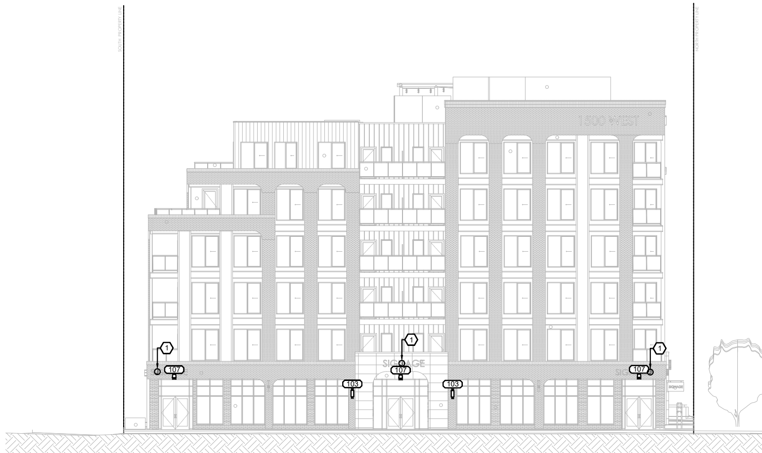
2 EAST BUILDING ELEVATION EXTERIOR LIGHTING LAYOUT SCALE: 1:250
