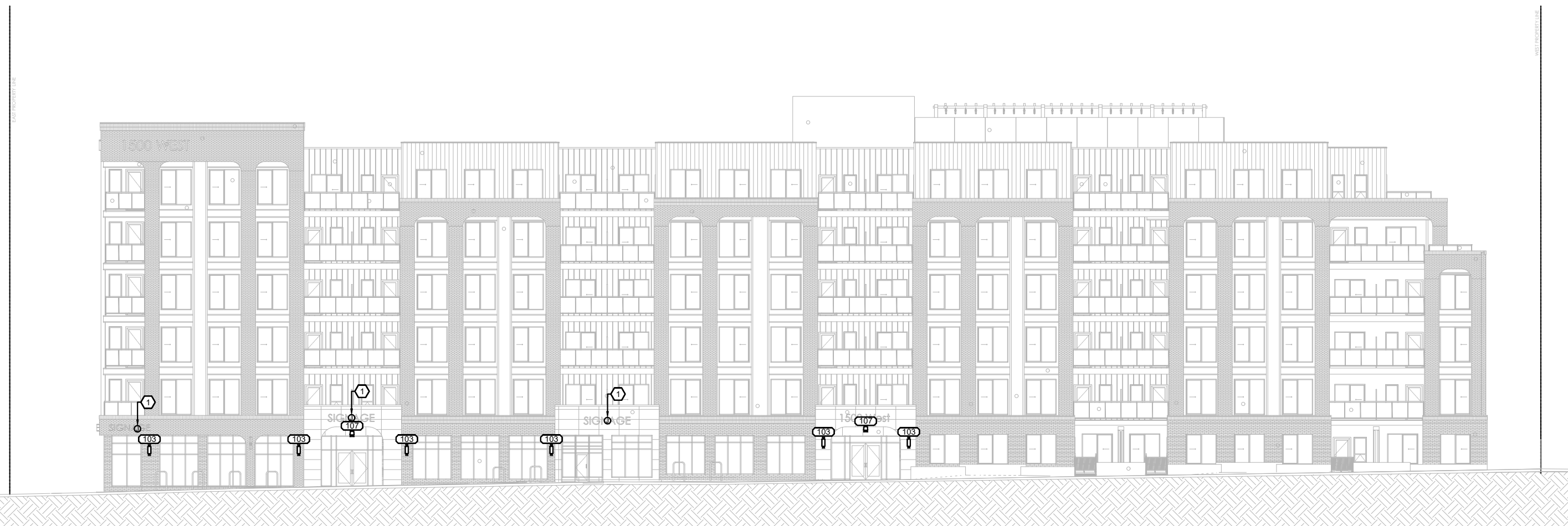
1 NORTH BUILDING ELEVATION EXTERIOR LIGHTING LAYOUT SCALE: 1:250
