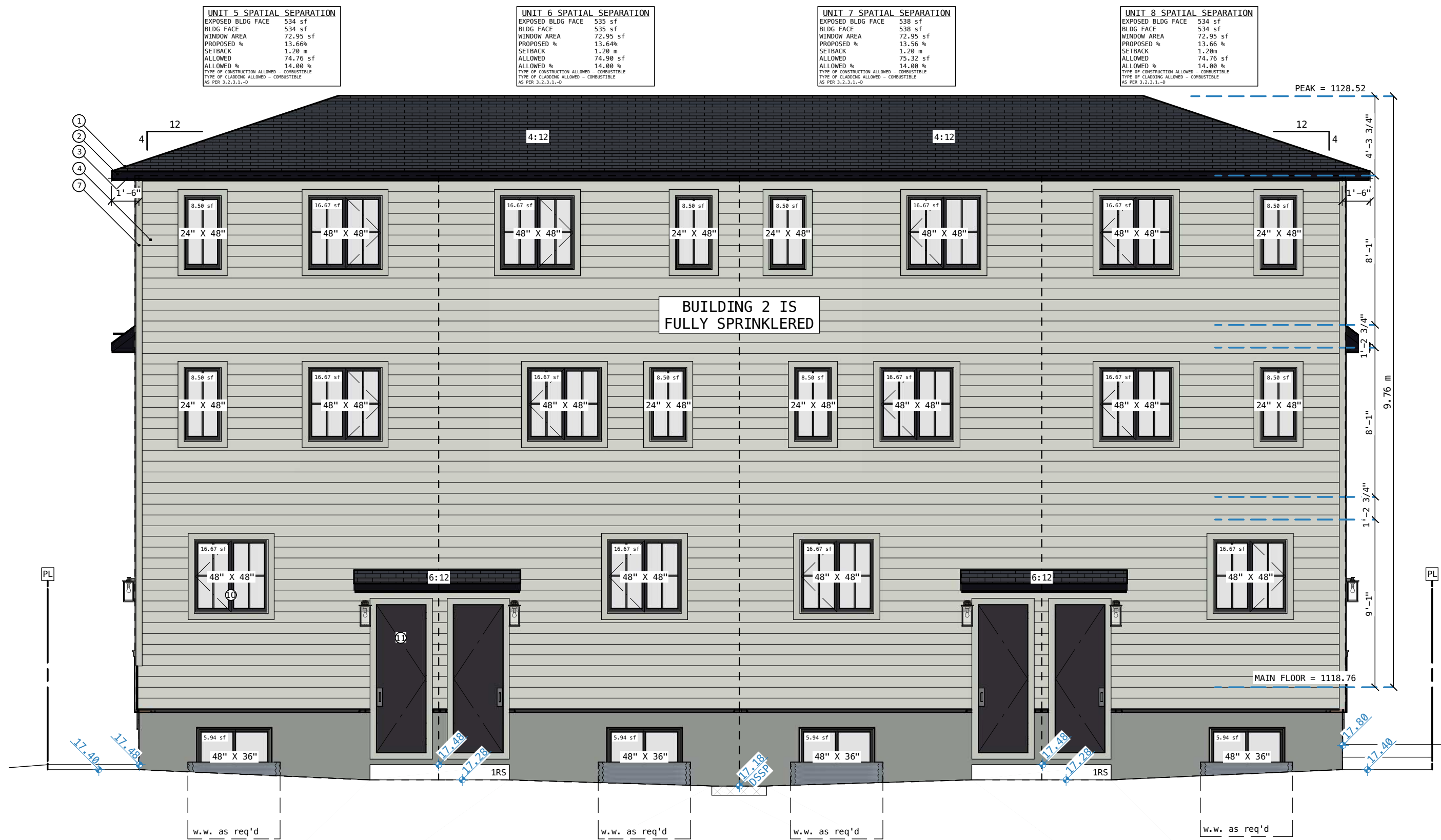
REAR ELEVATION – WEST – BUILDING 2 SCALE: 3/16"=1'-0"
