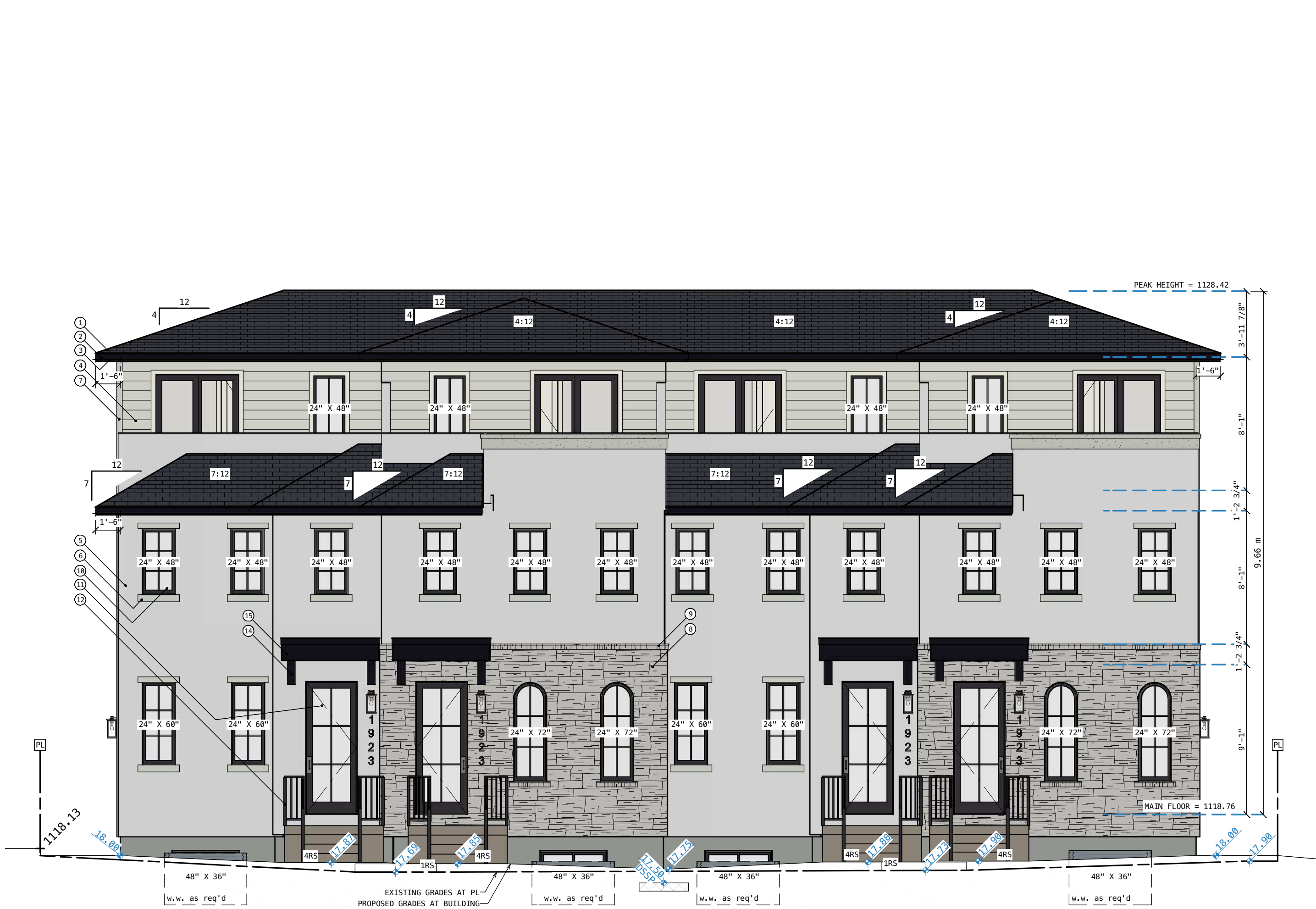
FRONT ELEVATION – EAST – BUILDING 1 SCALE: 3/16"=1'-0"
