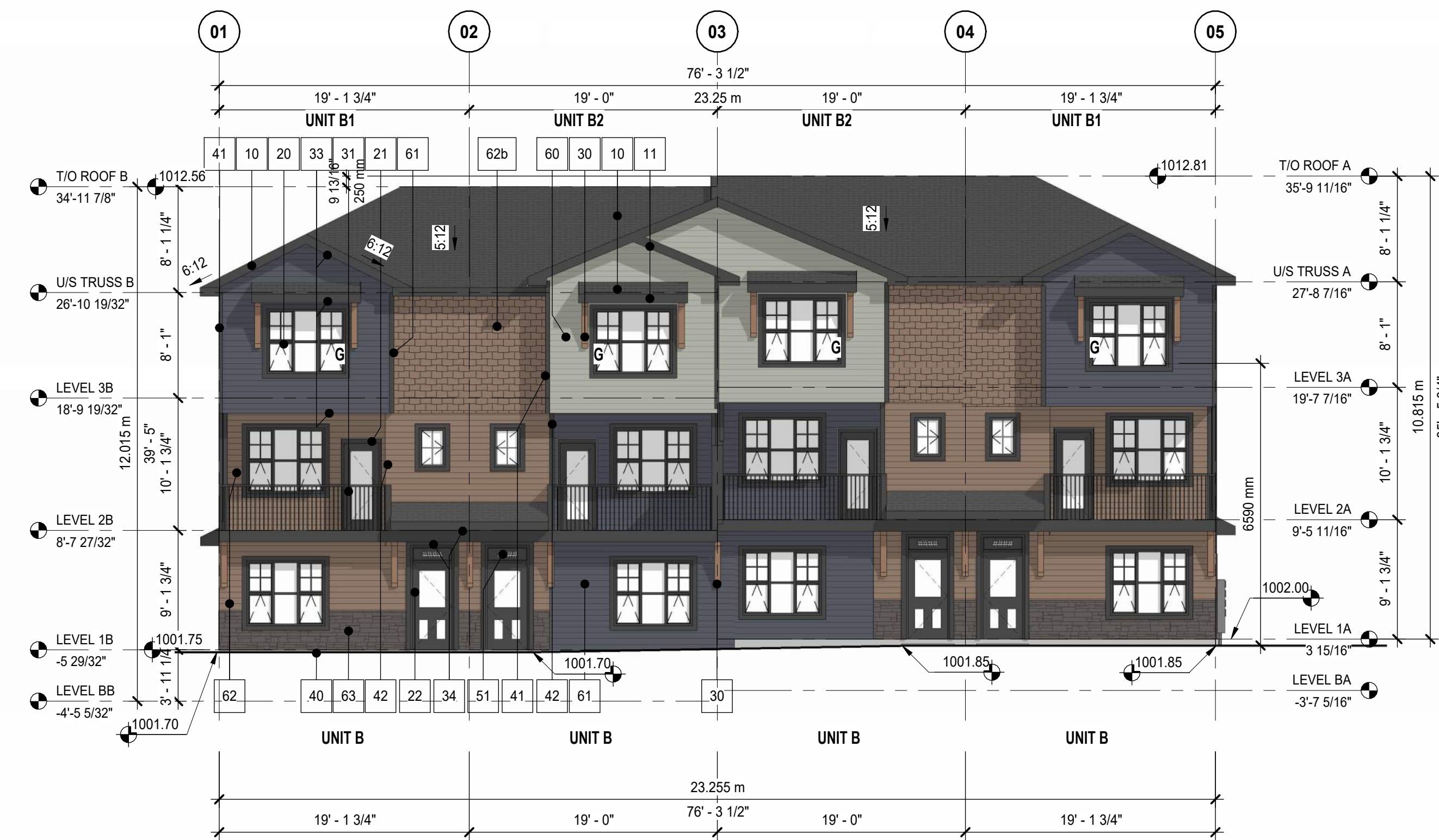
1 BLDG09 FRONT ELEVATION (NORTH-EAST) DP40-09-01 SCALE: 1/8" = 1'
