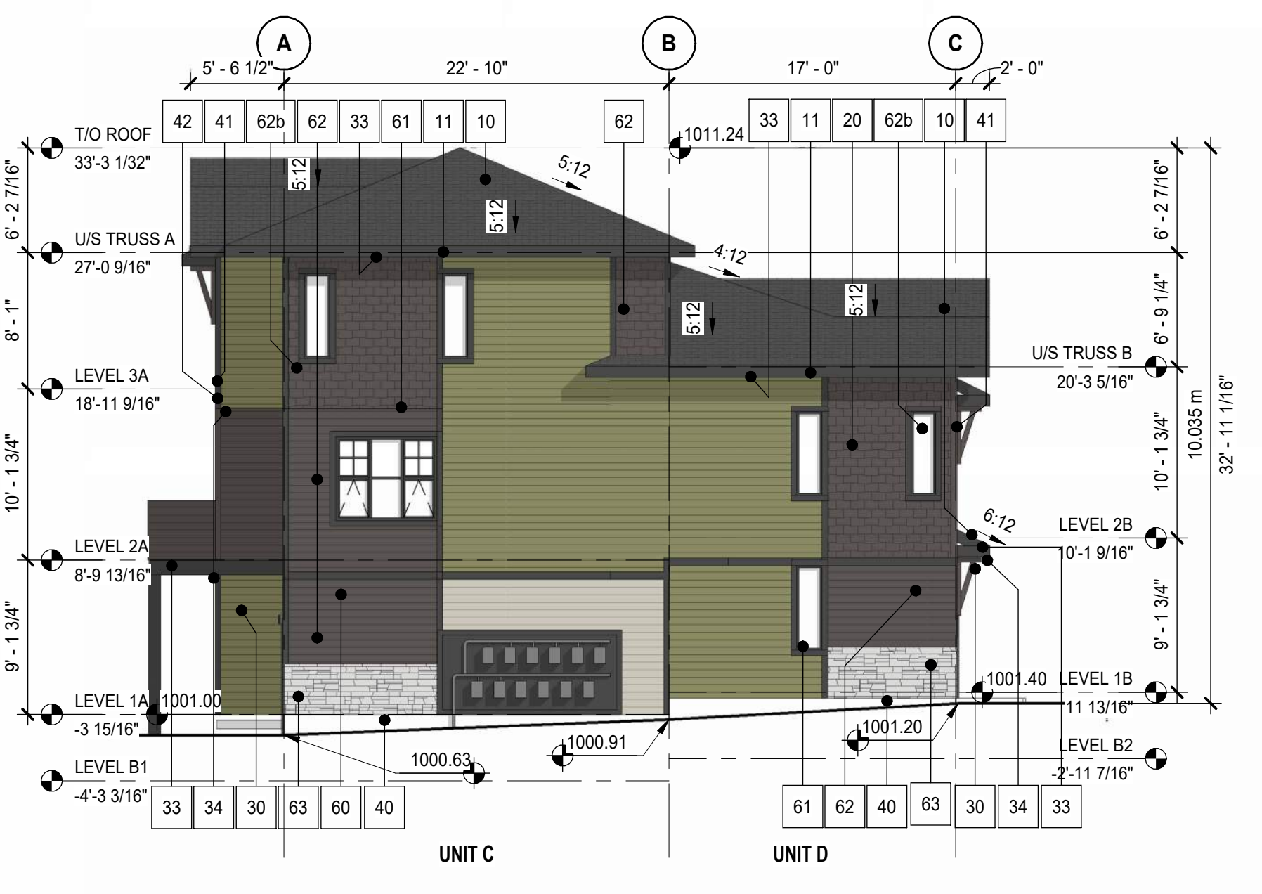
2 BLDG04 RIGHT ELEVATION (EAST) DP40-04-01 SCALE: 1/8" = 1'
