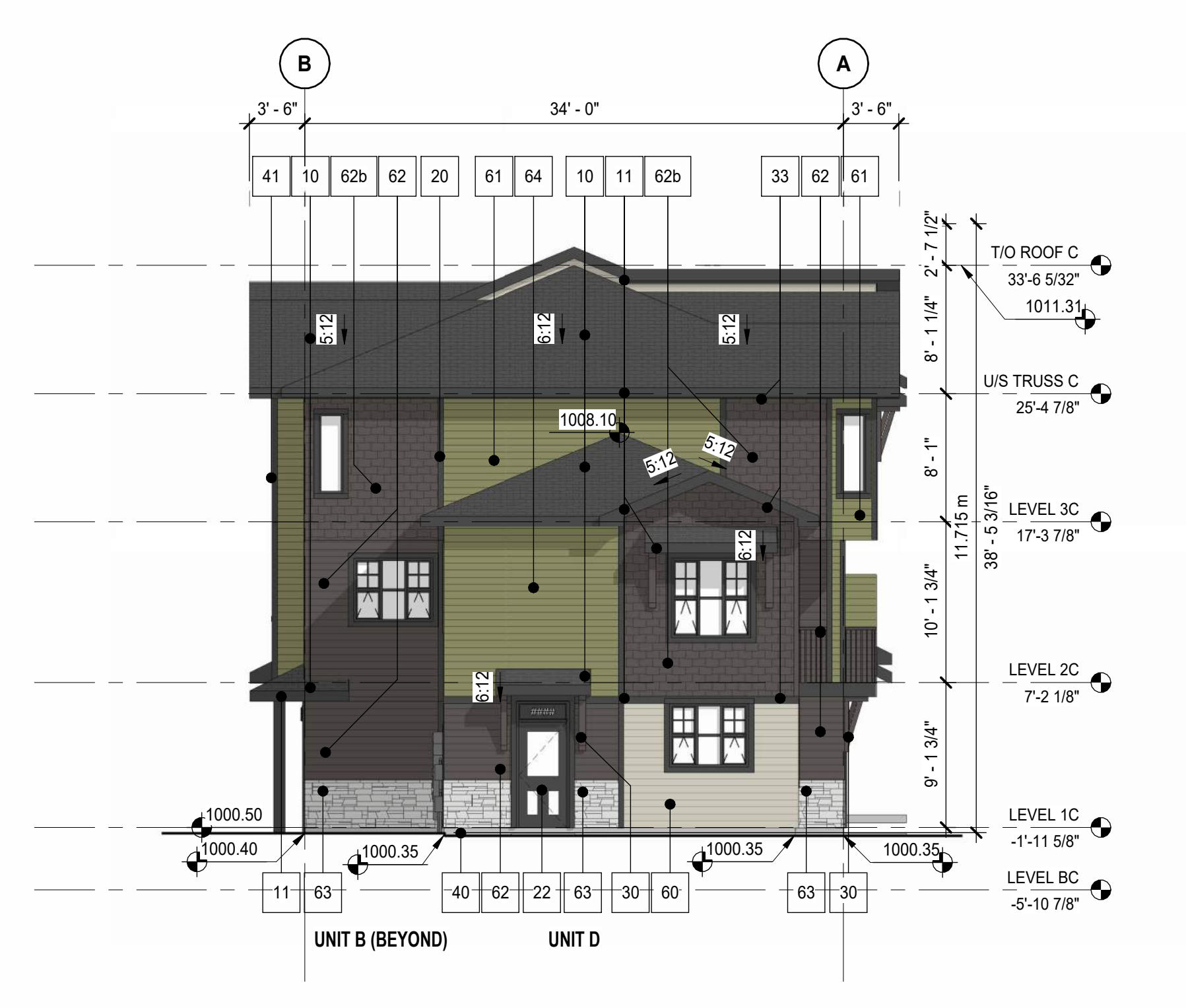
4 BLDG08 LEFT ELEVATION (SOUTH) DP40-08-01 SCALE: 1/8" = 1'
