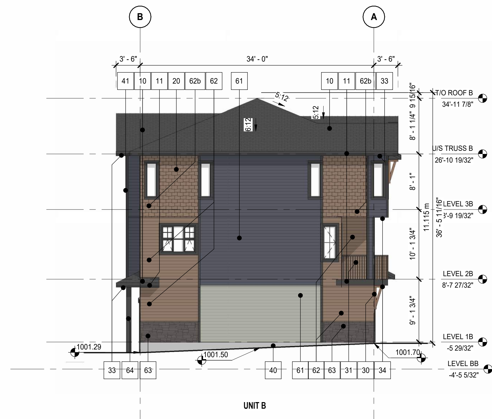
4 BLDG09 LEFT ELEVATION (SOUTH-EAST) DP40-09-01 SCALE: 1/8" = 1'
