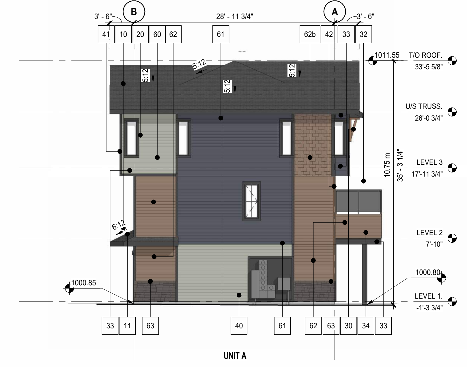
4 BLDG05 LEFT ELEVATION (WEST) DP40-05-01 SCALE: 1/8" = 1'
