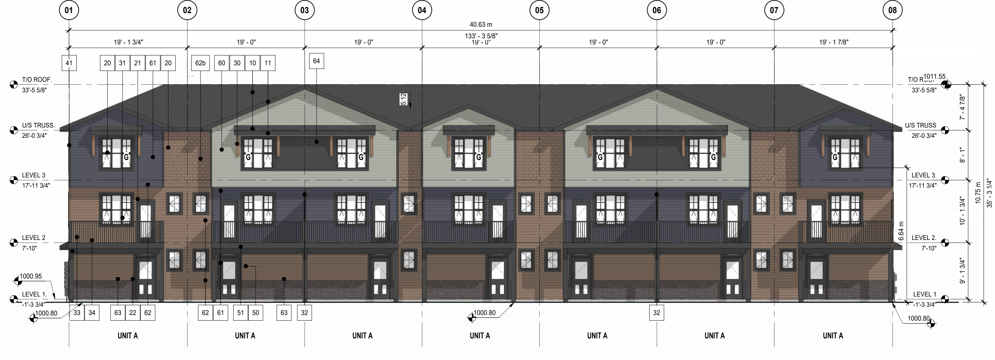
1 BLDG05 FRONT ELEVATION (SOUTH) DP40-05-01 SCALE: 1/8" = 1'
