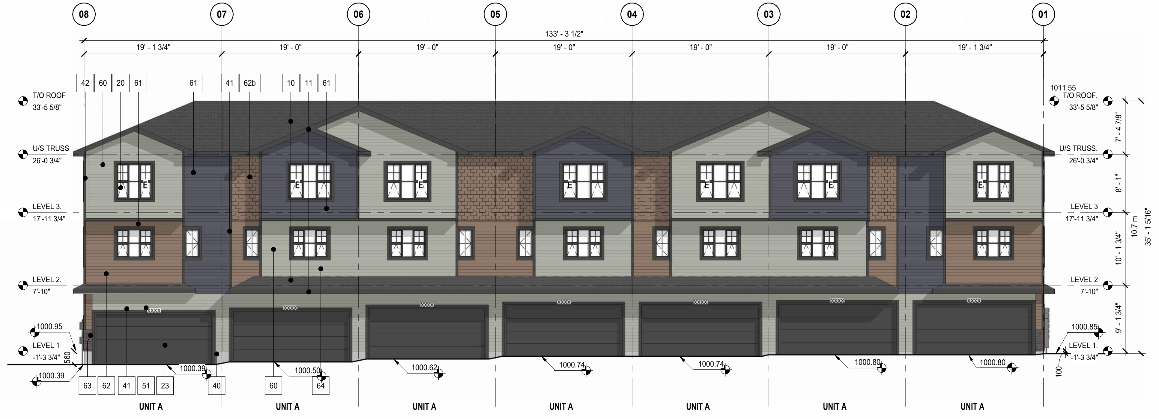
3 BLDG05 REAR ELEVATION (NORTH) DP40-05-01 SCALE: 1/8" = 1'
