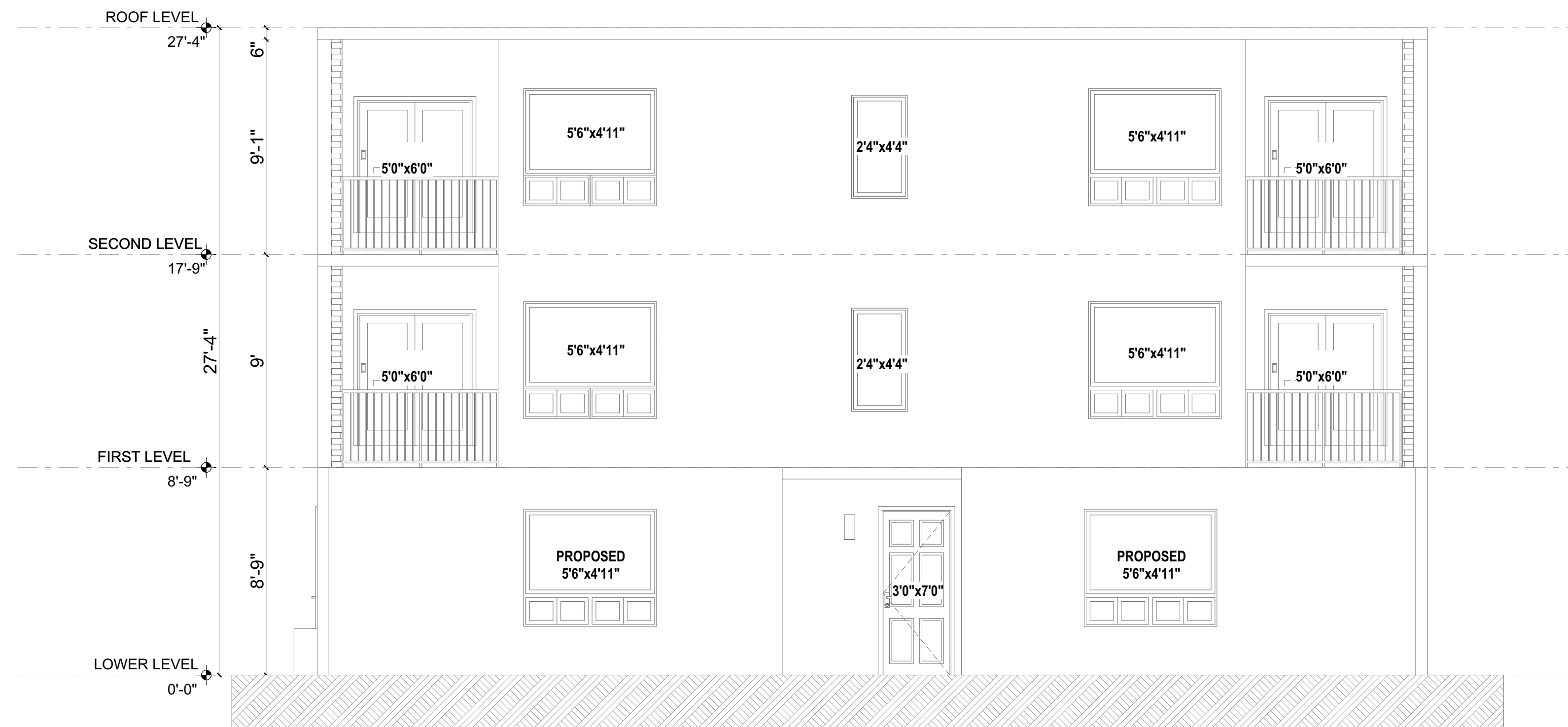
PROPOSED REAR ELEVATION SCALE: 1/4" : 1'-0"
