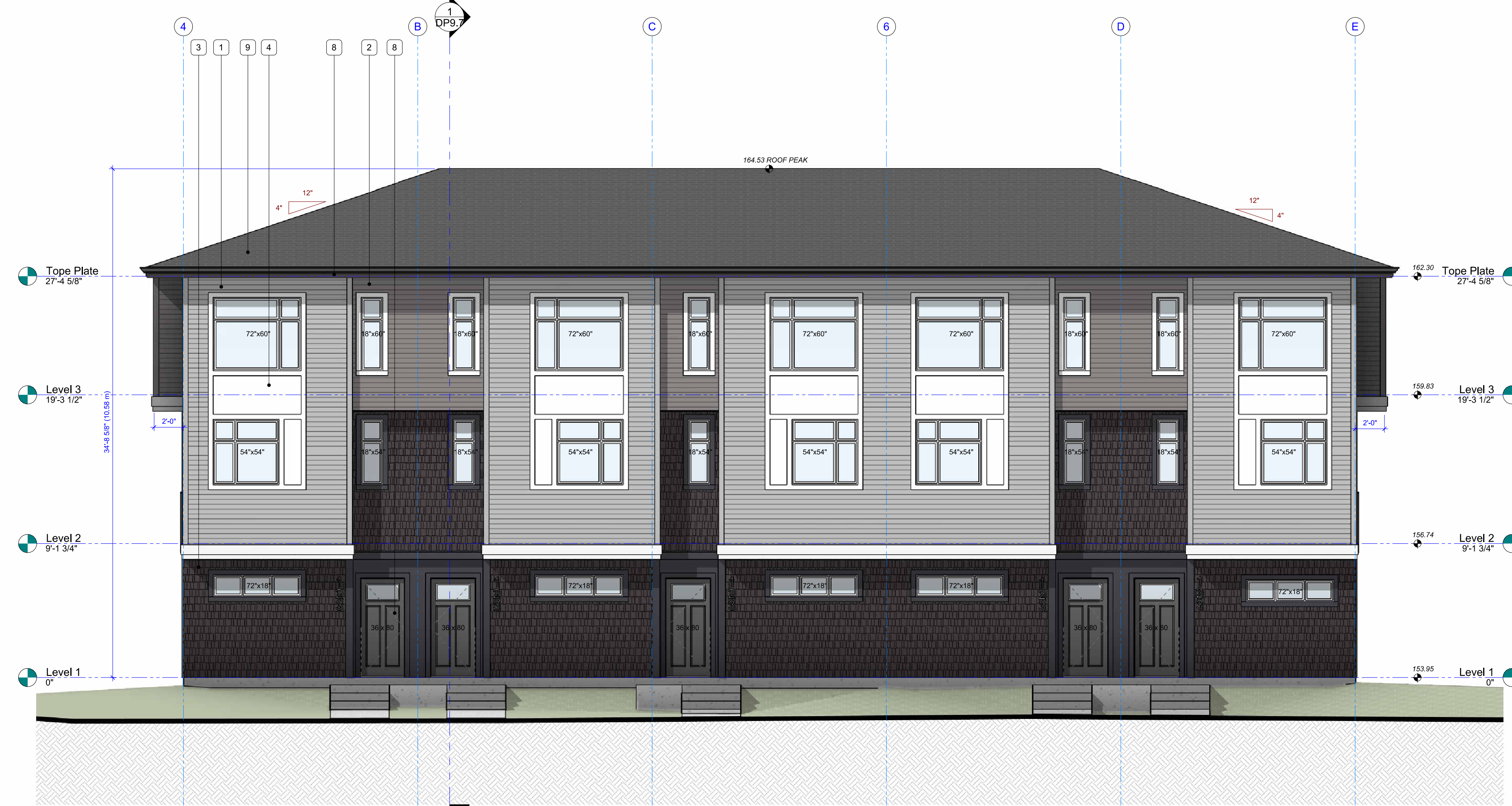
1 East Elevation (Bldg. 1 - Type F) 1 : 64
