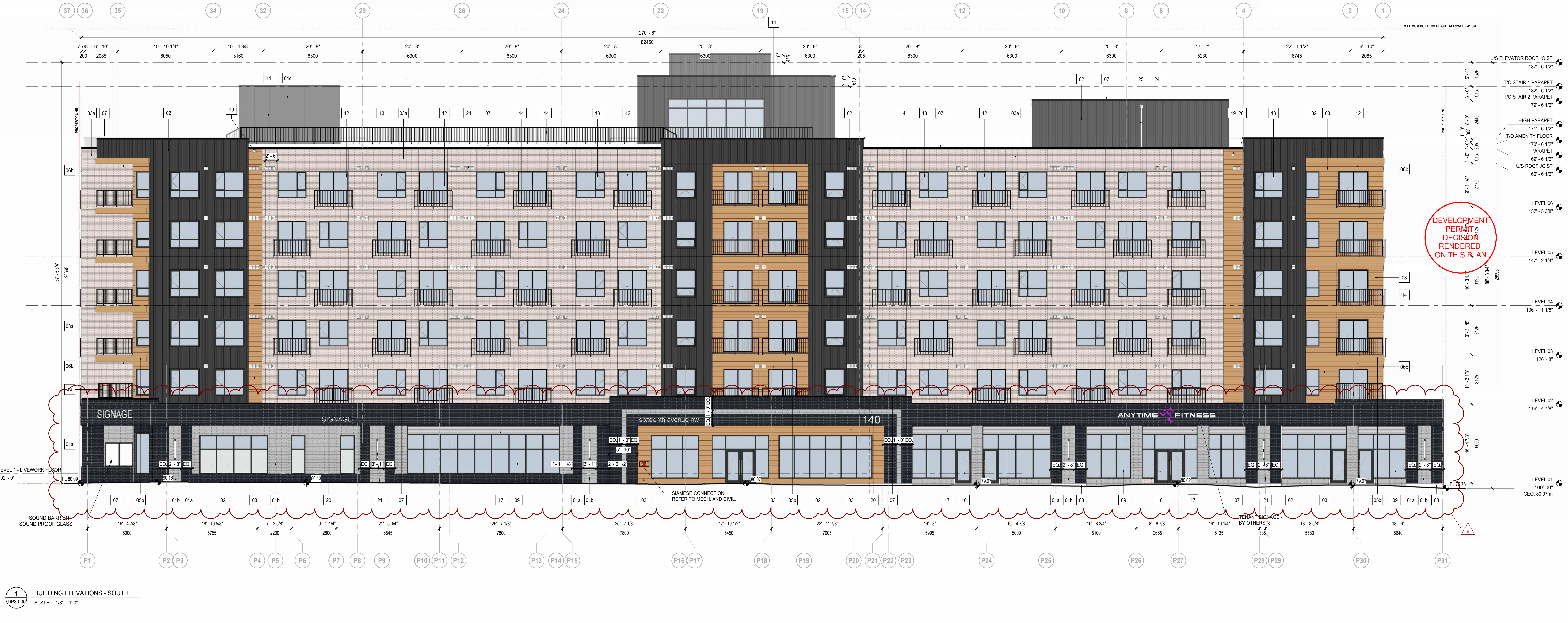
3 BUILDING ELEVATIONS - WEST WING SCALE: 1/8" = 1'-0"
