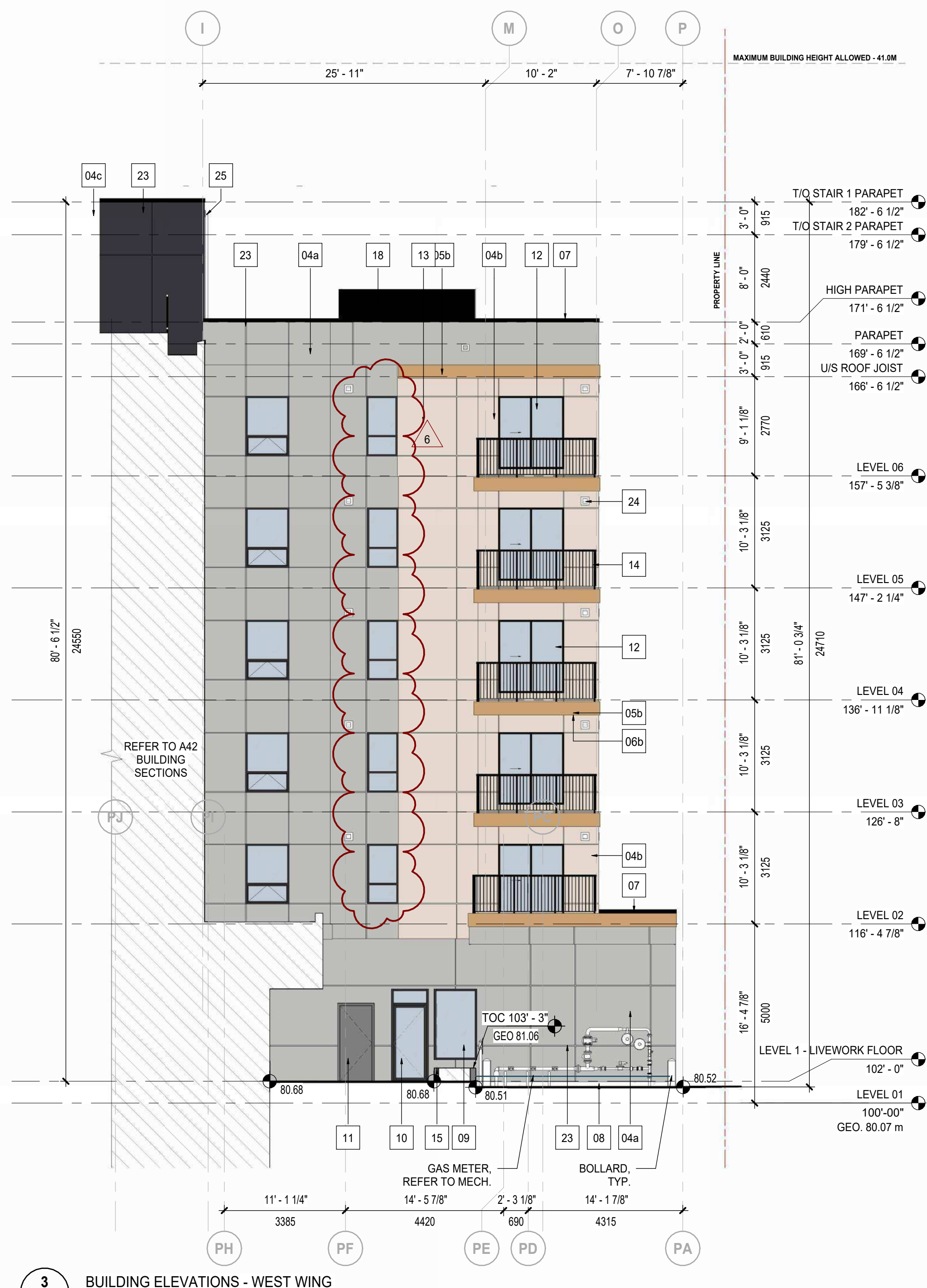
3 BUILDING ELEVATIONS - WEST WING SCALE: 1/8" = 1'-0"
