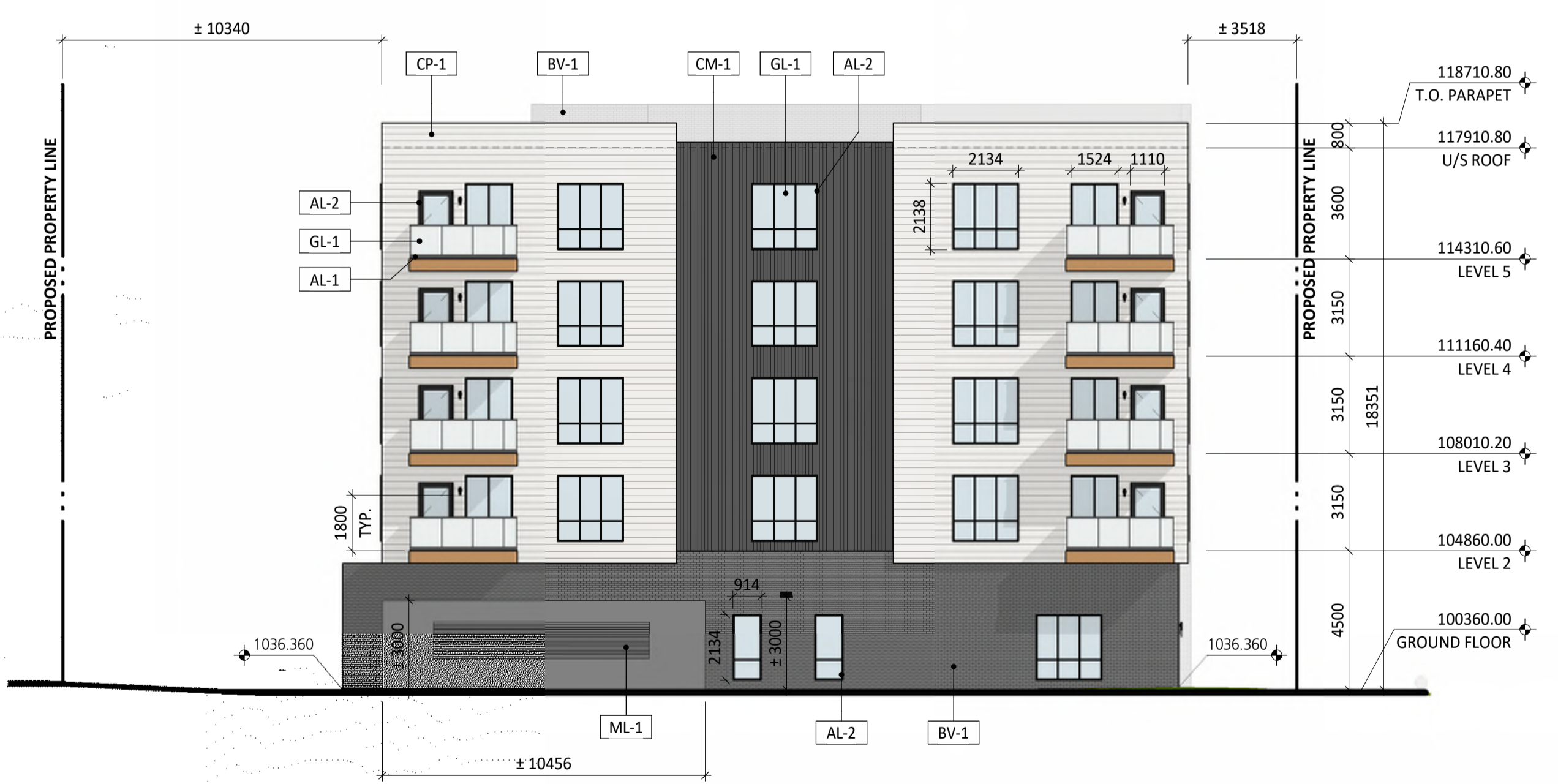
2 B2-SOUTH ELEVATION DP40.06 1 : 150
