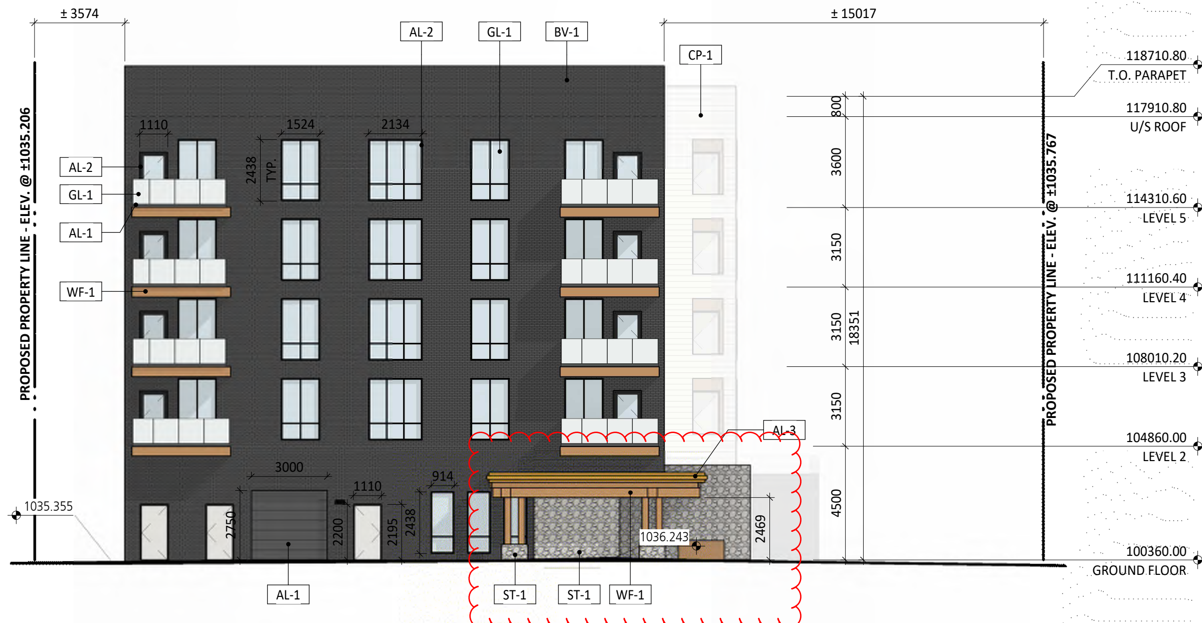
2 B2-NORTH ELEVATION DP40.05 1:150
