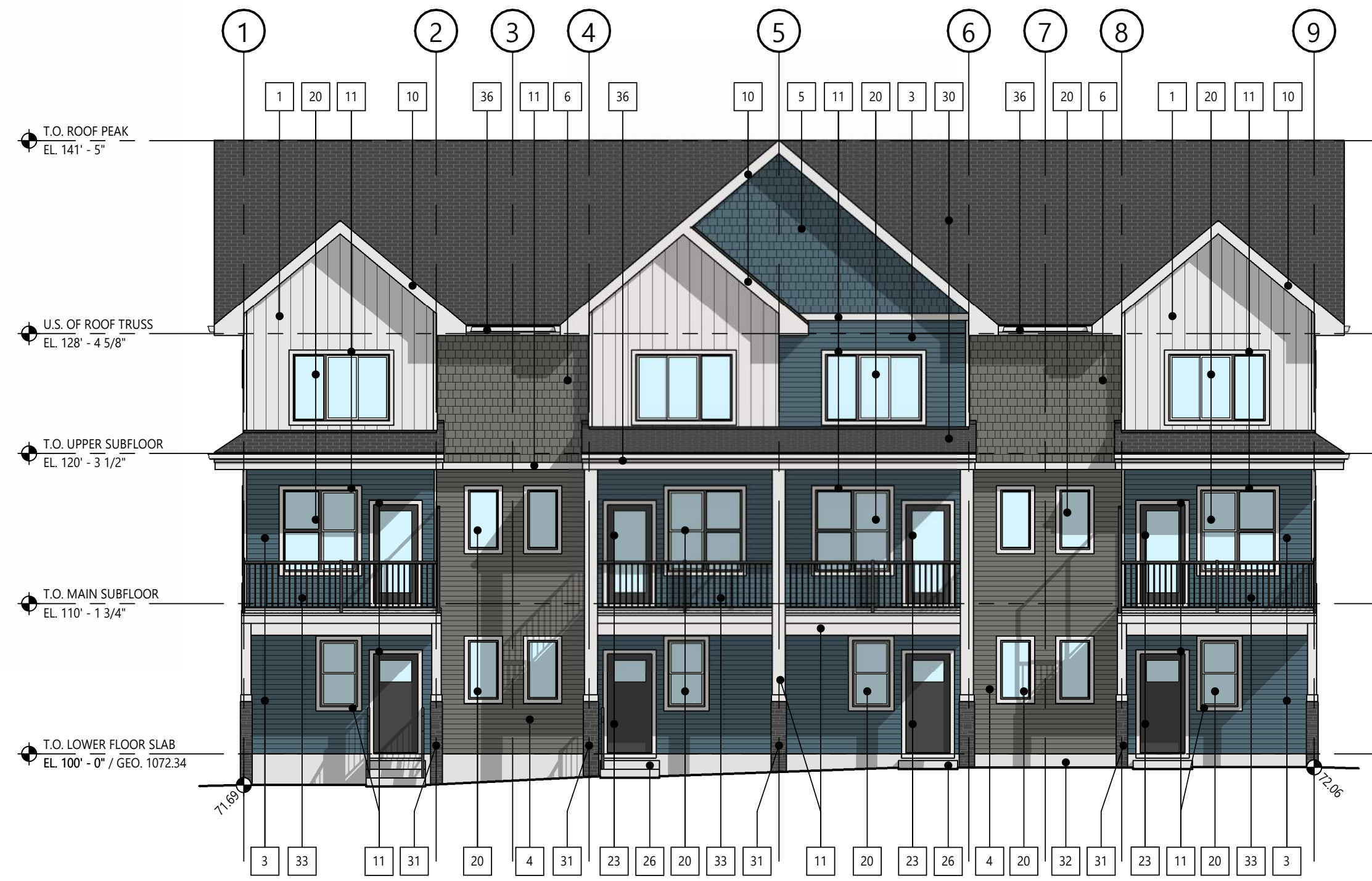
1 | BUILDING 12 - WEST ELEVATION DP4.10 SCALE: 1/8" = 1'-0"
