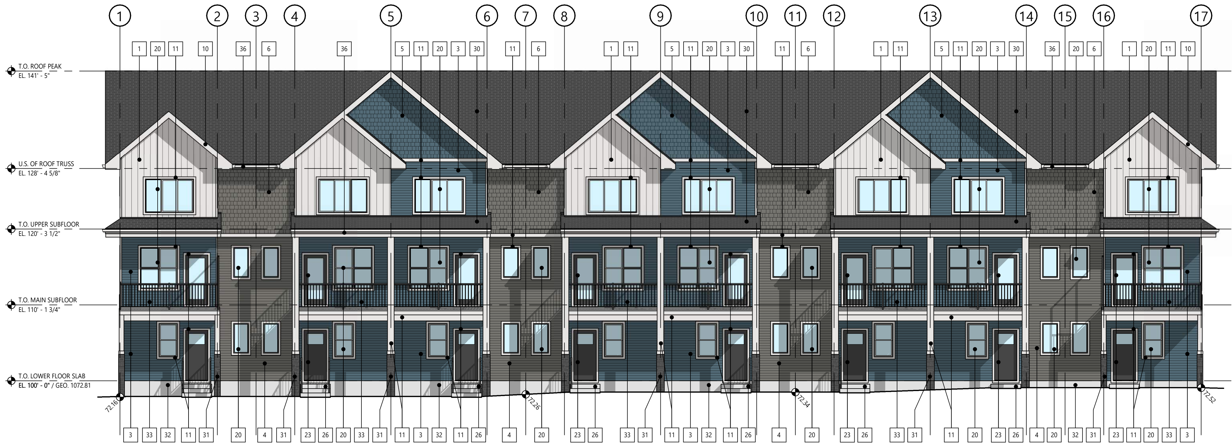
1 | BUILDING 13 - WEST ELEVATION DP4.11 | SCALE: 1/8" = 1'-0"
