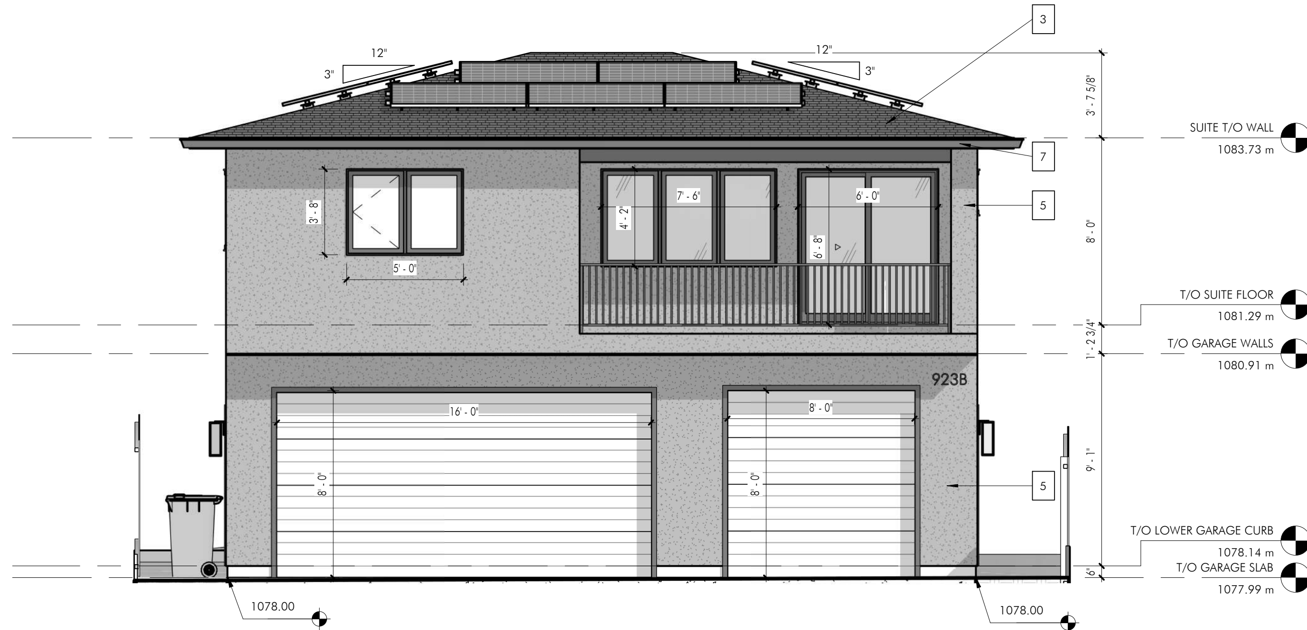
2 GARAGE - REAR ELEVATION 1/4" = 1'-0"
