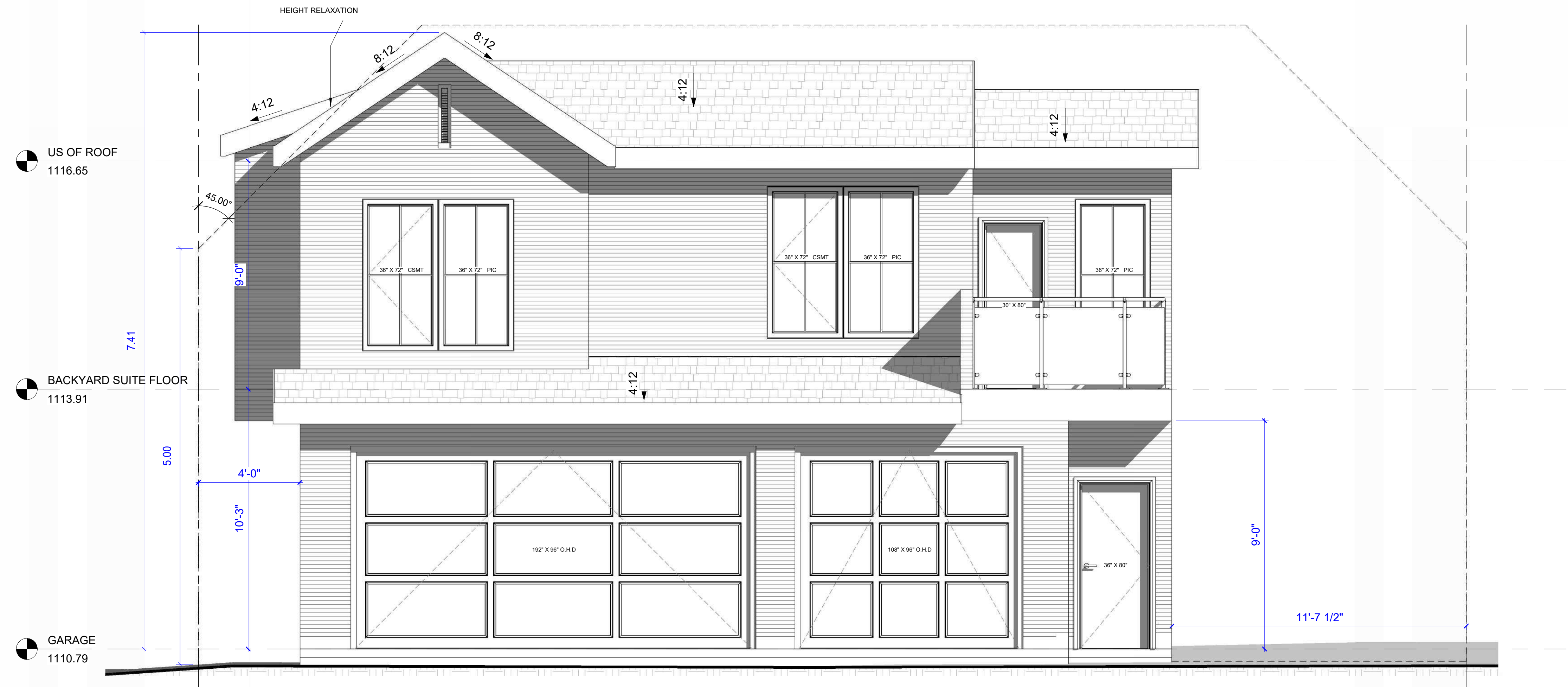
BACKYARD SUITE FRONT ELEVATION 3/8" = 1'-0"
