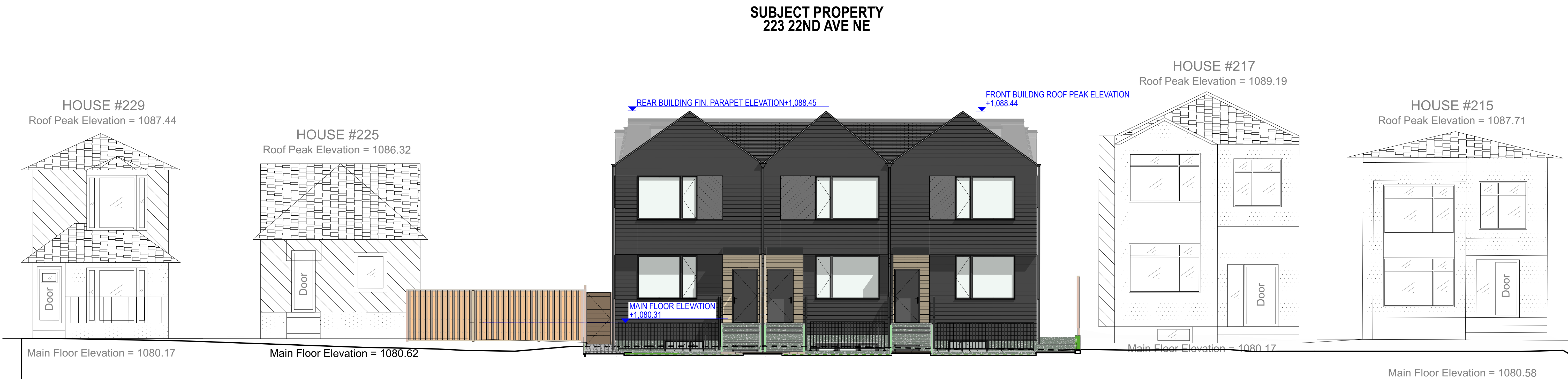
2 NORTH ELEVATION - STREETSCAPE SCALE: 1:75
