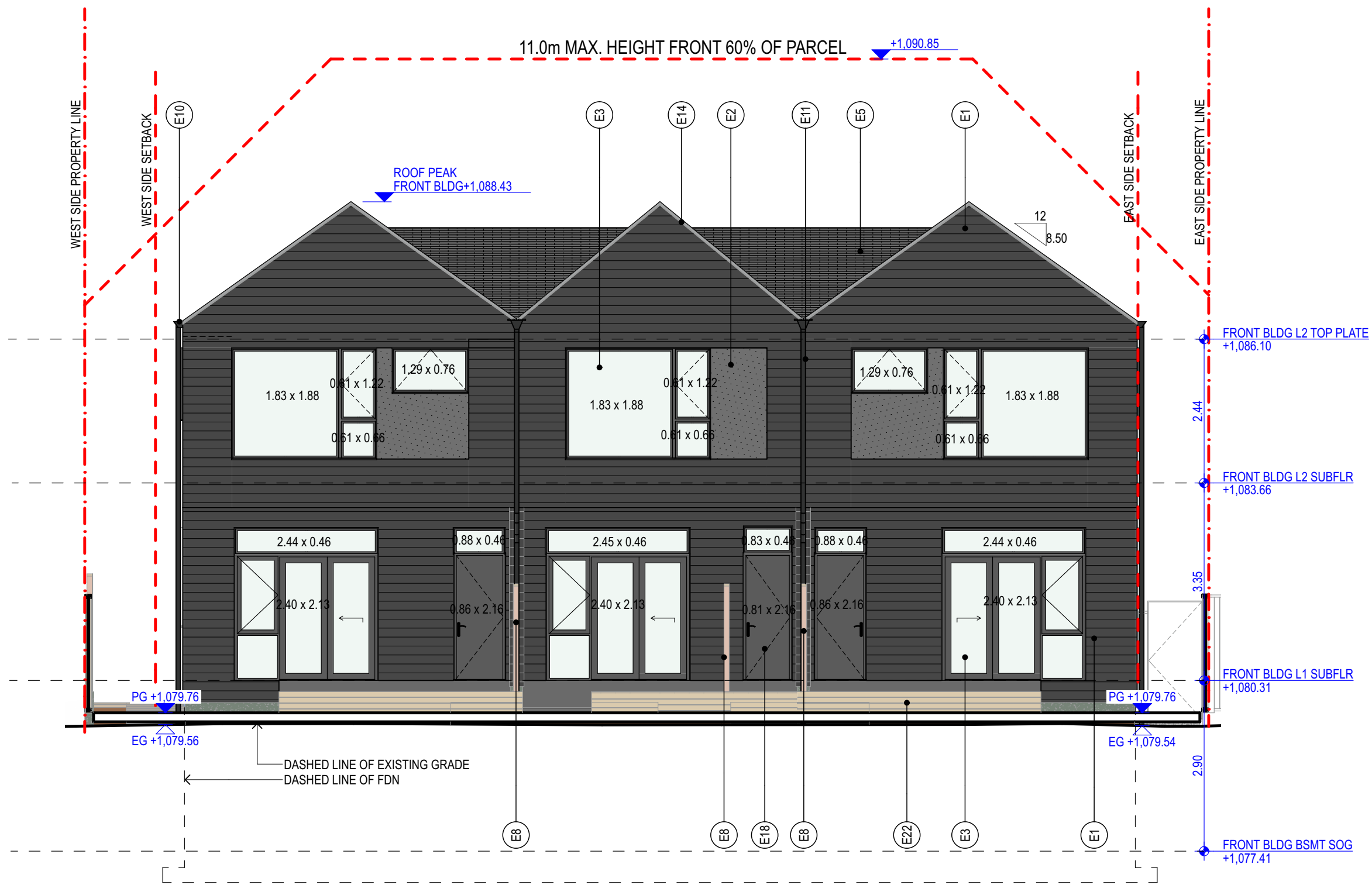
1 S1 SOUTH ELEVATION - FRONT BLDG SCALE: 1:75
